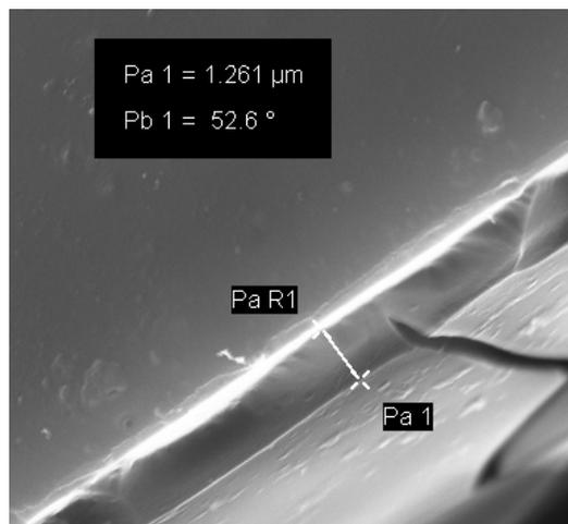
**Figure S8.** Cross sectional view of FESEM image of orange emitting film prepared via standard dip coating method.
