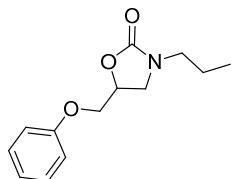
Synthesised according to General Experimental Procedure E using glycidyl phenyl ether (135 µL) and 1-propylamine (82 µL), and purified by flash column chromatography (25% EtOAc/Petroleum ether 40 – 60 °C) and strong cation exchange chromatography (MeOH) to afford the title compound as a clear oil (101 mg, 58%).
