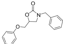
Synthesised according to General Experimental Procedure E using glycidyl phenyl ether (135  $\mu$ L) and benzylamine (109  $\mu$ L), and purified by flash column chromatography (30% EtOAc/Petroleum ether 40 – 60 °C) to afford the title compound as a white solid (266 mg, 94%).
