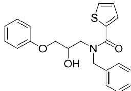
Synthesised according to General Experimental Procedure C using glycidyl phenyl ether (135  $\mu$ L), benzylamine (109  $\mu$ L) and ethyl 2-thiophenecarboxylate (134  $\mu$ L), and purified by flash column chromatography (30% EtOAc/Petroleum ether 40 – 60 °C) and strong cation exchange chromatography (MeOH) to afford the title compound as a yellow oil (218 mg, 59%).
