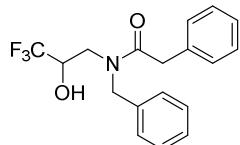
Synthesised according to General Experimental Procedure C using 2-(trifluoromethyl)oxirane (86 µL), benzylamine (109 µL) and methyl phenylacetate (140 µL), and purified by flash column chromatography (20% EtOAc/Petroleum ether 40 – 60 °C) and strong cation exchange chromatography (MeOH) to afford the title compound as a pale yellow oil (233 mg, 69%).
