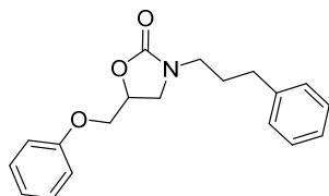
Synthesised according to General Experimental Procedure E using glycidyl phenyl ether (135 µL) and 3-phenylpropylamine (142 µL), and purified by flash column chromatography (25% EtOAc/Petroleum ether 40 – 60 °C) and strong cation exchange chromatography (MeOH) to afford the title compound as a white solid (134 mg, 43%).
