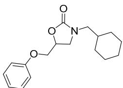
Synthesised according to General Experimental Procedure E using glycidyl phenyl ether (135 µL) and cyclohexylmethylamine (130 µL) and purified by flash column chromatography (35% EtOAc/Petroleum ether 40 – 60 °C) to afford the title compound as a pale yellow solid (255 mg, 88%).
