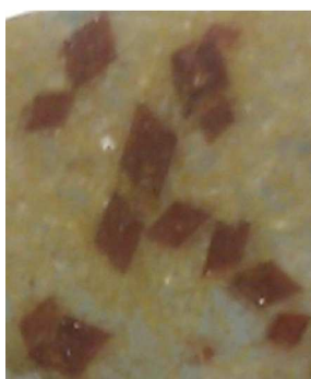
Figure S1. Prismatic crystals ( ca. 2 mm on an edge (left), and acicular crystals ( ca. 0.2 \times 0.2 \times 0.7 mm) of compound 1 (right). Acicular crystals had well-developed (101), (-1\ 0\ 1) , \pm(110) , \pm(-1\ 1\ 0) , \pm(010) , \pm(011) , \pm(1\ -1\ 1) , \pm(1\ -1\ 0) , \pm(100) and \pm(001) faces.
