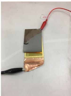
**Figure S2.** The optical images of EPD chamber. (a) left: top electrode, right: bottom chamber electrode, (b) EPD chamber, which is connected with wires (the top electrode is applied positive voltage and the bottom chamber is applied ground.)
