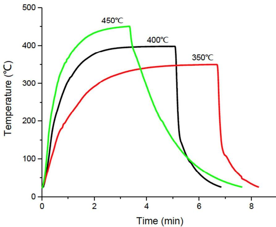
Figure 1. Temperature profiles in proxy reactors with highest water vol% loading for different sand bath set point temperatures
