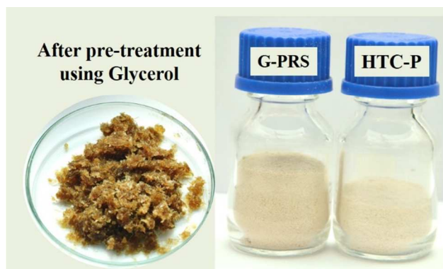
Figure S1. Photographs of RAW-P , RAW-P after pre-treatment in glycerol ( G-PRS ) and chitin ( HTC-P )
