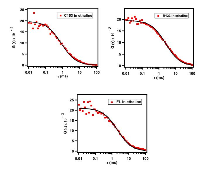
**Figure S4.** Fluorescence correlation curves for the diffusion of solutes in ethaline. The points are the experimental data and the solid lines represent fit to the data using single component diffusion model. The excitation wavelengths are 405 nm for C153 and 485 nm for R123 and FL.
