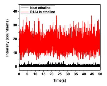
**Figure S2.** Fluorescence intensity time trace of ethaline alone and R123 in ethaline ( $\lambda_{exc} = 485$  nm).
