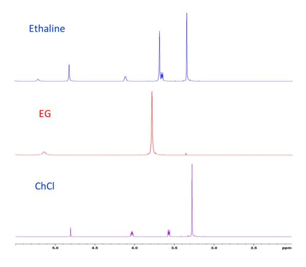
**Figure S1.** <sup>1</sup>H-NMR spectra of choline chloride (ChCl), ethylene glycol (EG) and ethaline (CD<sub>3</sub>OD as reference).
