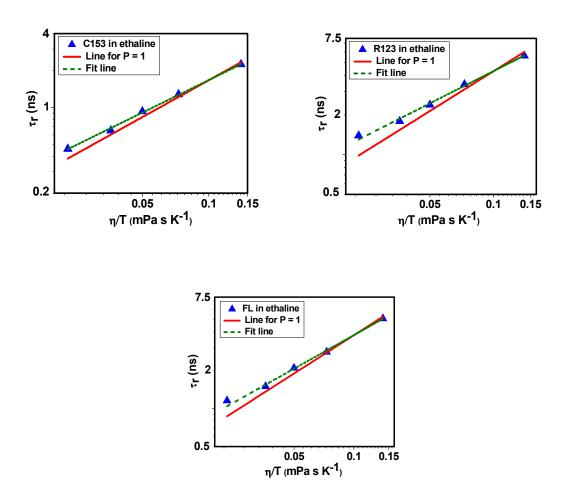
Fig. S6: Dependence of the  $\tau_r$  values of C153, R123 and FL in ethaline on  $\eta/T$  according to  $\tau_r = A(\eta/T)^P$  shown as dashed lines. The hypothetical line with P=1 is shown as solid line.
