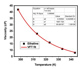
**Figure S3.** Measured viscosity (points) of ethaline at different temperatures together with the fits (solid line) ccording to the Vogel–Fulcher–Tamman (VFT) equation.
