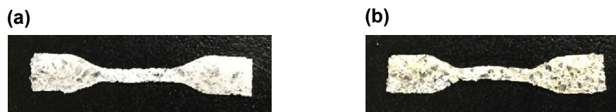
Figure S7. Photographs of (a) P(HMA-co-ADSA) and (b) P(HMA-co-HDA) after the reprocessing procedure for 48 h.
