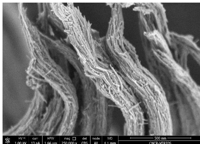
**Figure S3.** SEM image of a nanocast  $\text{Co}_3\text{O}_4$  “replica” synthesized using a distorted/corrugated SBA-15 as the template.
