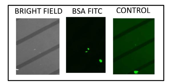
Figure S-2. FITC BSA is used to determine the degree of detachment of immobilized P selectin after flow experiment. Control is the device without P selectin immobilization and treated with FITC BSA. It shows the non-specific attachment in terms of fluorescence. The device after the flow experiment (middle figure) shows no fluorescence and hence P selectin is intact after flow experiment which is important for proper device operation.
