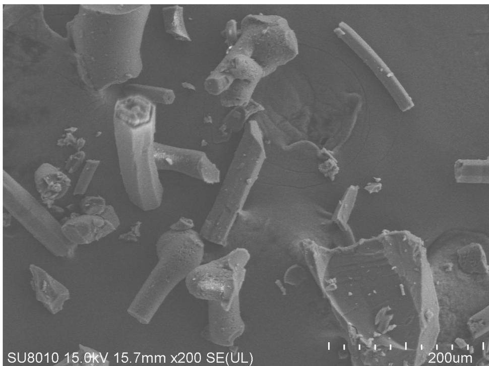
**Figure S27.** Scanning electron microscopy image of  $I_2@EtP6$  crystalline solids after iodine release in cyclohexane.
