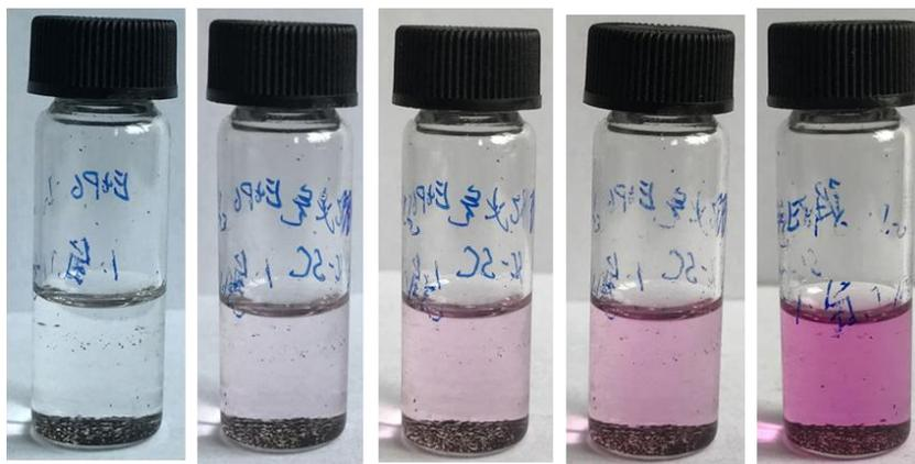
**Figure S32.** Photographs showing the color change of cyclohexane (2 mL) upon addition of  $I_2@EtP6$  single crystals. The color change is due to the iodine release from  $I_2@EtP6$  single crystals.
