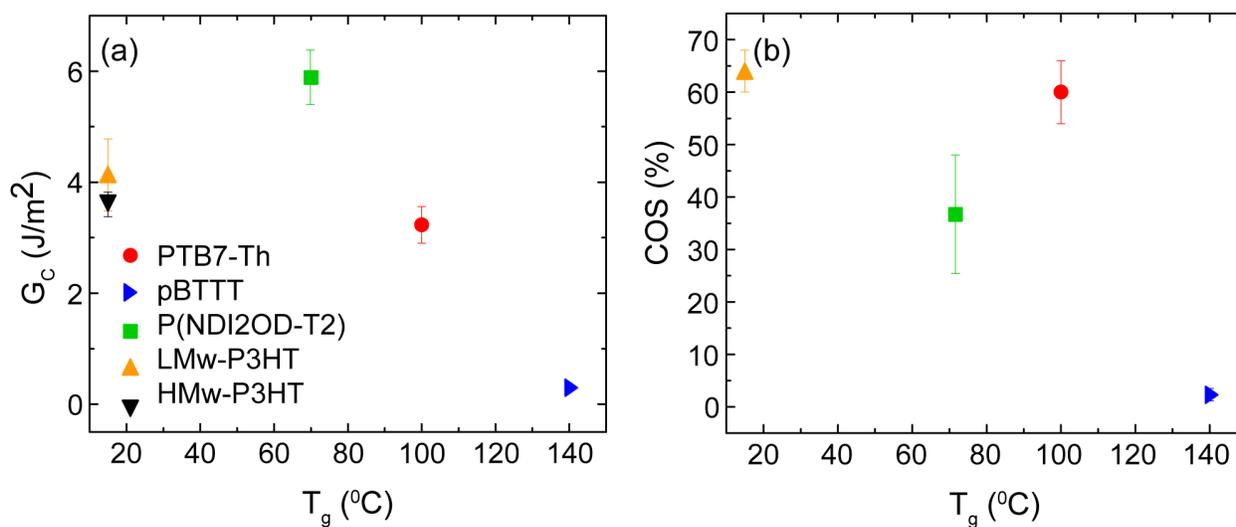
**Figure S4.** (a) Cohesive fracture energy and (b) crack onset strain (COS) of the polymer films at their estimated glass transition temperatures ( $T_g$ ). All properties are reported for  $100 \pm 25$  nm thick films.
