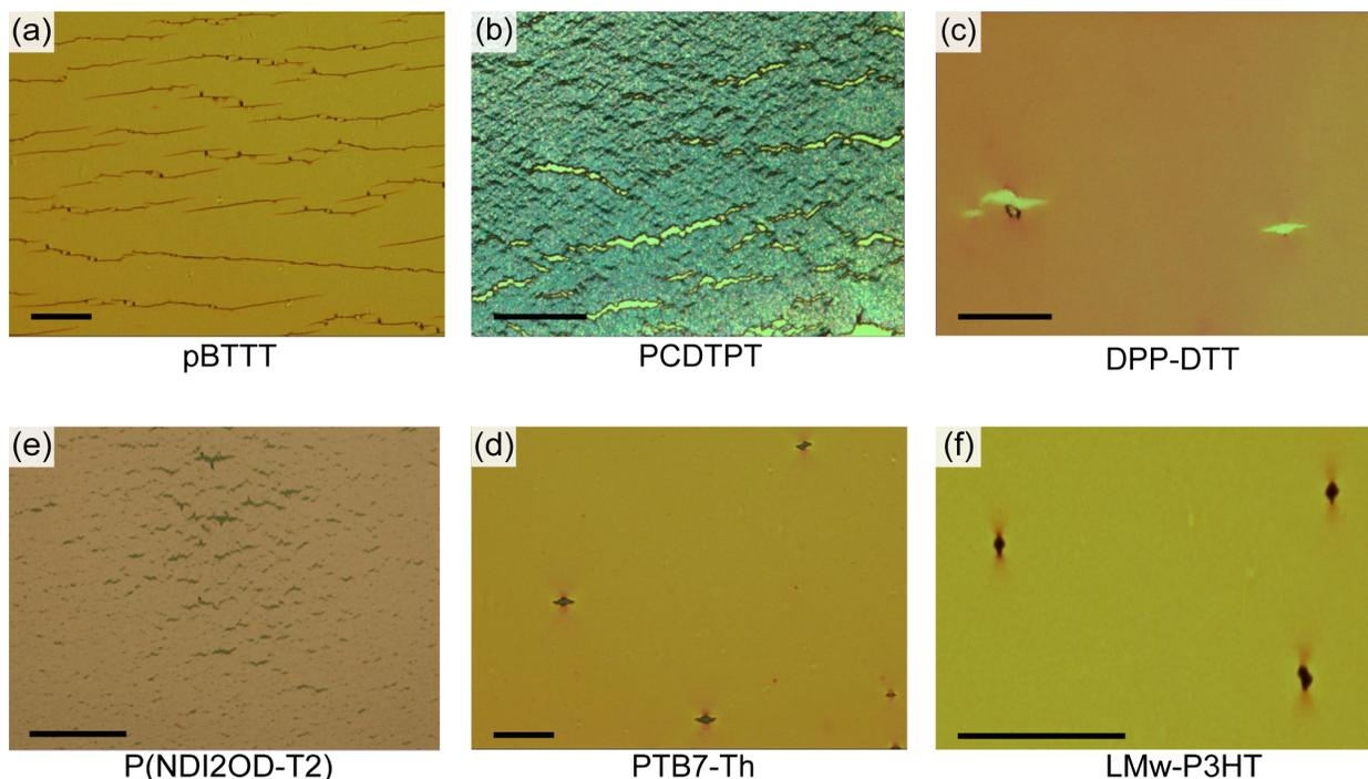
**Figure S3.** Optical microscopic images of characteristic crack features observed in the COS measurements for (a) pBTTT, (b) PCDTPT, (c) DPP-DTT, (d) P(NDI2OD-T2), (e) PTB7-Th, and (f) LMw-P3HT films. All images were captured near their respective crack onset strains. In all films, the strain was applied along the long axis of the page. The scale bar for all images is 50  $\mu\text{m}$ .
