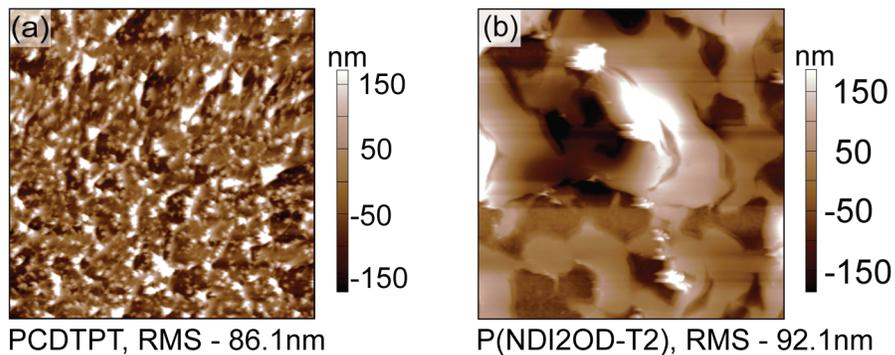
**Figure S2.** AFM height images for the fractured film surfaces. The films are (a) 268 nm thick PCDTPT film which exhibited fracture energy of  $1.09 \text{ J/m}^2$  and (b) 116 nm thick P(NDI2OD-T2) film which exhibited fracture energy of  $5.89 \text{ J/m}^2$ .
