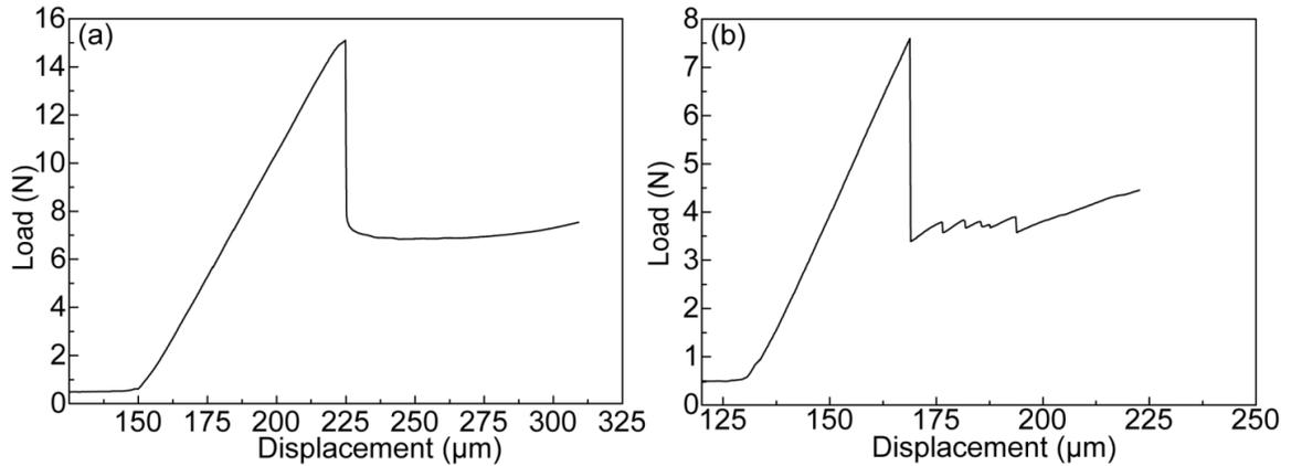
**Figure S1.** Load vs. displacement profile exhibiting (a) a smooth plateau corresponding to PTB7-TH indicative of stable crack propagation and (b) a saw-tooth profile in the plateau corresponding to PCDTPT indicative of unstable crack propagation.
