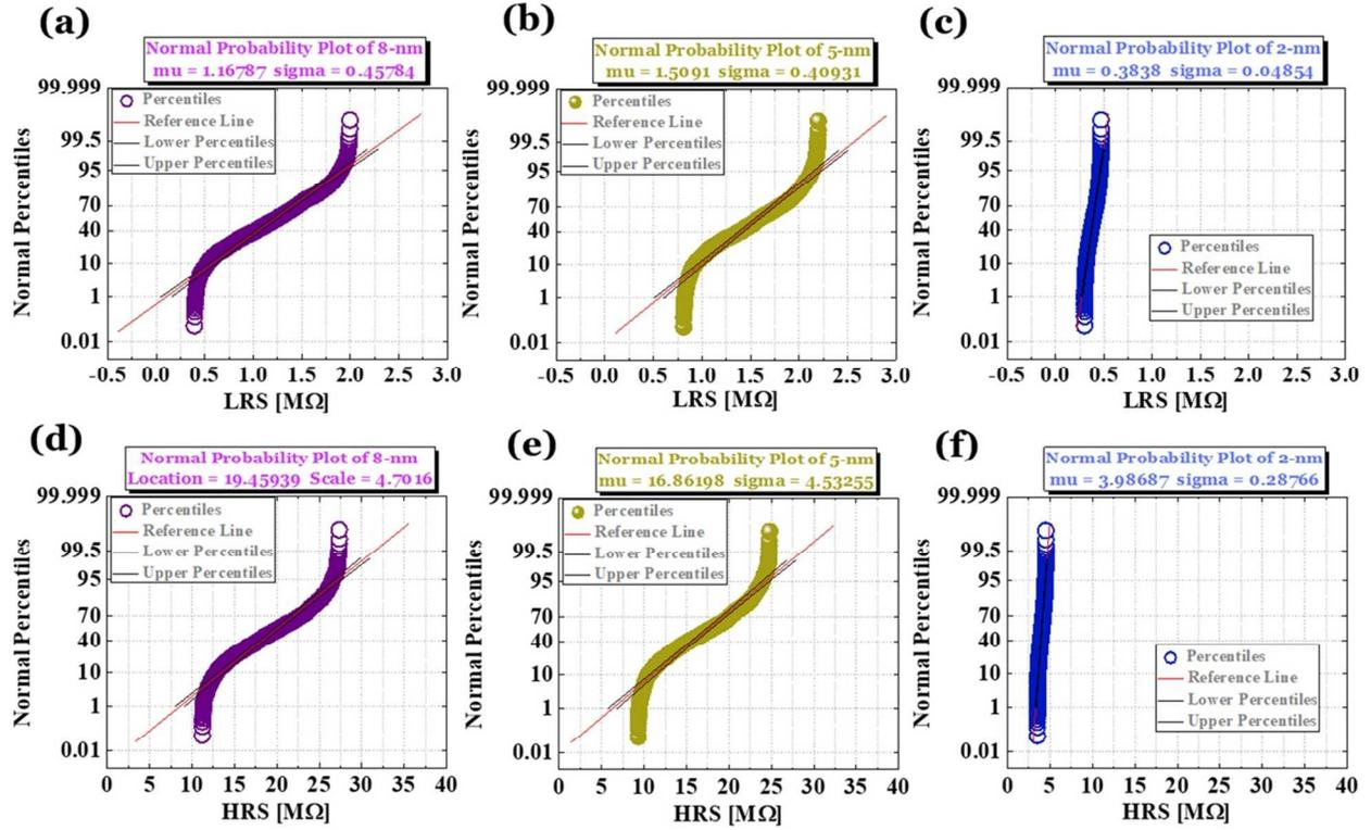
**Figure S3. Variation of LRS and HRS.** The cycle-to-cycle variation of the LRS for (a) S1, (b) S2, and (c) S3 devices, respectively. The cycle-to-cycle variation of the HRS for (d) S1, (e) S2, and (f) S3 devices, respectively. In all cases the controllability is improving the 2 nm  $\text{Al}_2\text{O}_3$  based RRAM device structure.
