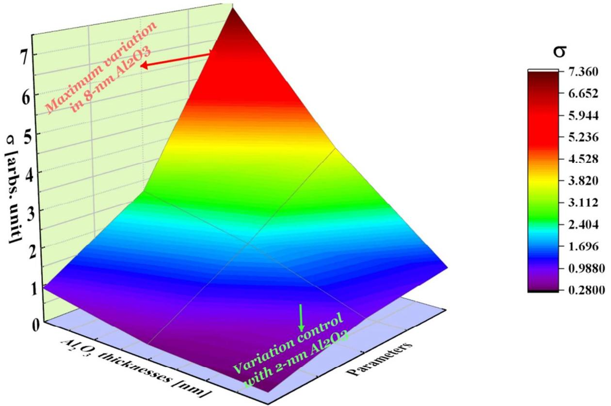
**Figure S4. Surface plot of variation.** The surface plot of variation is showing an excellent control of the variability by ultra-thin 2 nm  $\text{Al}_2\text{O}_3$  layer as compare to the thicker  $\text{Al}_2\text{O}_3$  layer.
