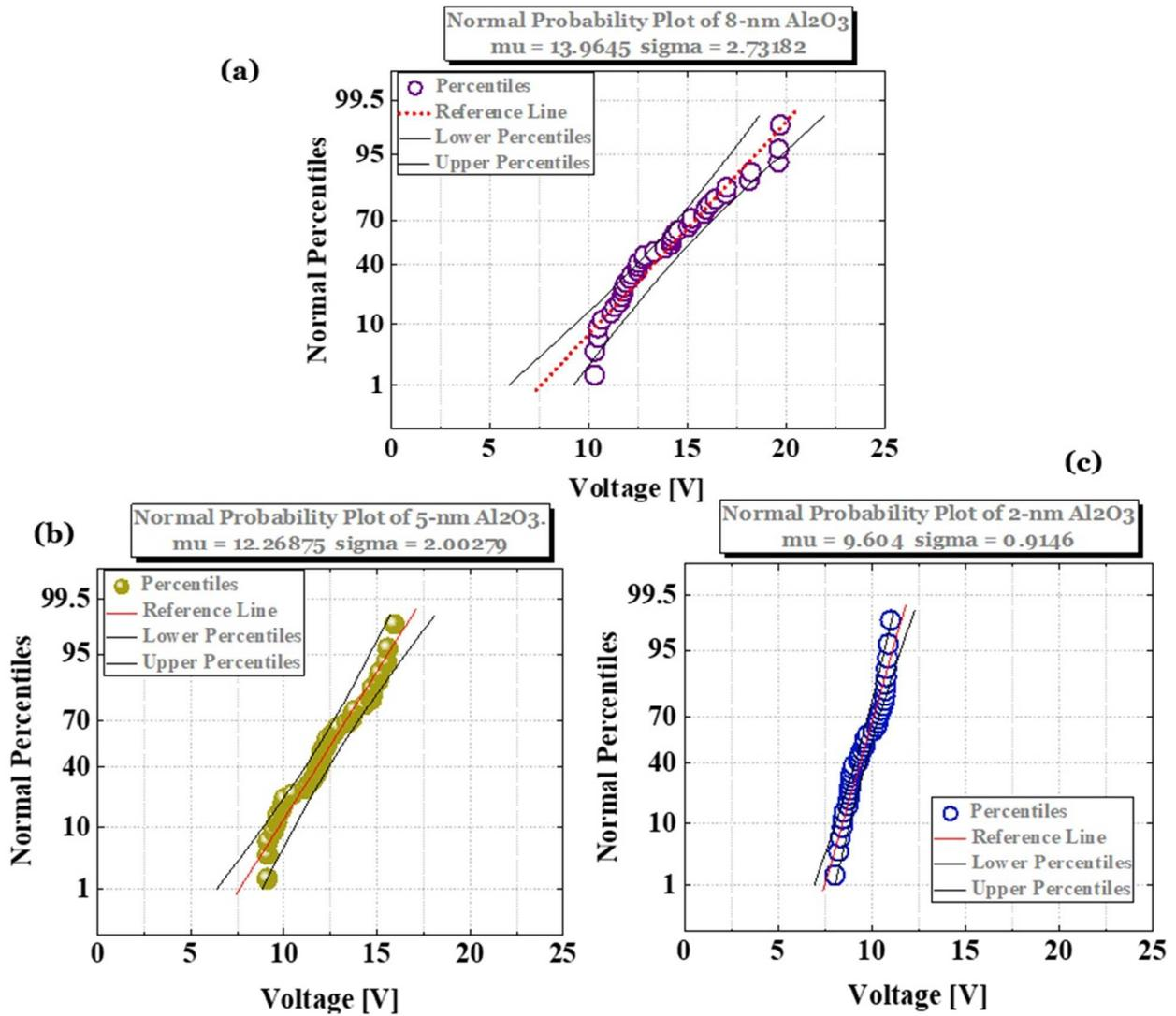
**Figure S1. Initial forming voltage distribution with different TiO<sub>x</sub>/Al<sub>2</sub>O<sub>3</sub> RRAM devices.** Device-to-device forming voltage distribution for (a) S1, (b) S2, and (c) S3 devices. Due to the thicker Al<sub>2</sub>O<sub>3</sub> layer, the S1 devices need higher voltage as compare to the S3 devices.
