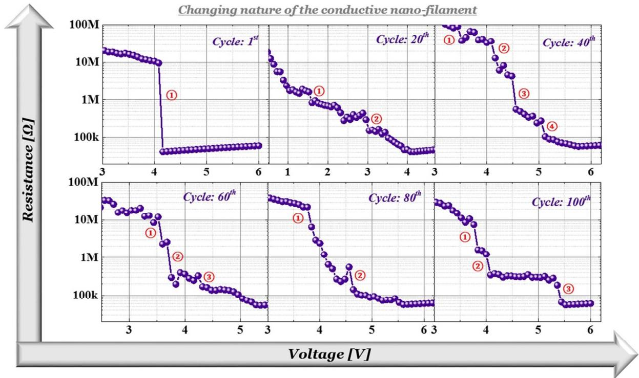
**Figure S2. Transition from HRS to LRS in S1 RRAM devices.** The cycle-to-cycle transition from HRS to LRS is showing a non-uniform evolution of CNF. Due to that the variation in resistive switching cycles are obvious.
