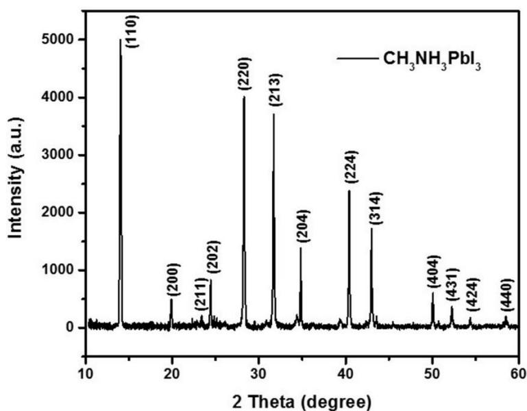
Figure S3. XRD pattern of  $\text{CH}_3\text{NH}_3\text{PbI}_3$  perovskite on glass substrate.
