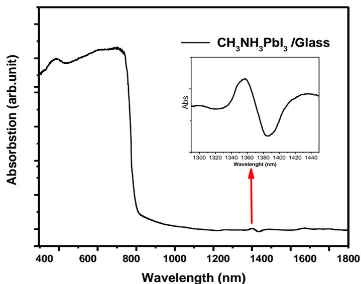
Figure S2. The absorption spectra of  $\text{CH}_3\text{NH}_3\text{PbI}_3$  perovskite on glass substrate.
