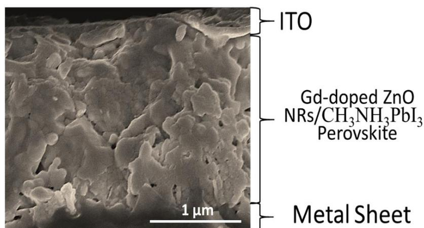
Figure S1. Cross-sectional SEM images Gd-doped ZnO NRs/CH<sub>3</sub>NH<sub>3</sub>PbI<sub>3</sub>/ITO fabricated on 316L stainless steel.
