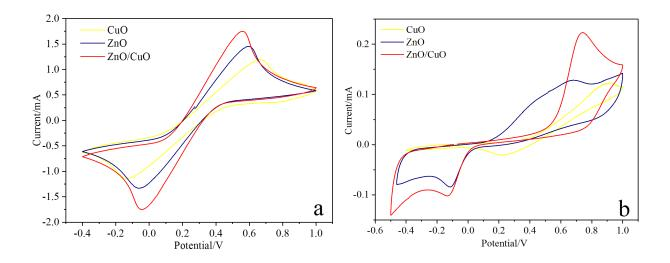
S6: CV curves of CuO, ZnO, and ZnO/CuO NTs in 1 mM  $\rm Fe(CN)_6^{3-}/\rm Fe(CN)_6^{4-}$  in 0.1 M KCl aqueous solution (a), and 1 mM ferrocene in 0.1 M BuNF<sub>4</sub> in acetonitrile (b).
