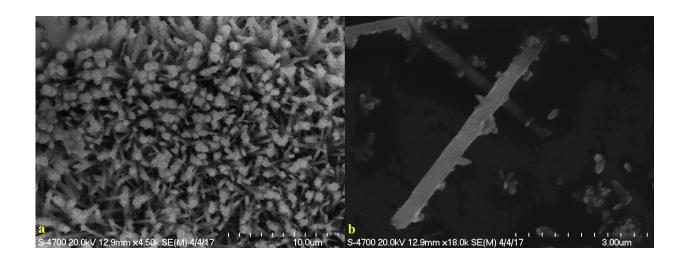
S1: SEM images of ZnO/CuO NTs (a) and a single ZnO/CuO NT (b).
