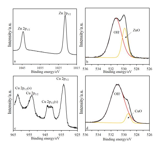
S3: XPS spectrum of Zn 2p  $(2p_{1/2}: 1044.45, 2p_{3/2}: 1021.35)$ , O 1s in ZnO nanowires (OH<sup>-</sup>: 531.25, ZnO: 529.85), Cu 2p  $(2p_{1/2}(s): 962.07, 2p_{1/2}: 954.97, 2p_{3/2}(s): 941.37, 2p_{3/2}: 933.57)$ , and O 1s in CuO nanorods (OH<sup>-</sup>: 531.97, CuO: 529.37).
