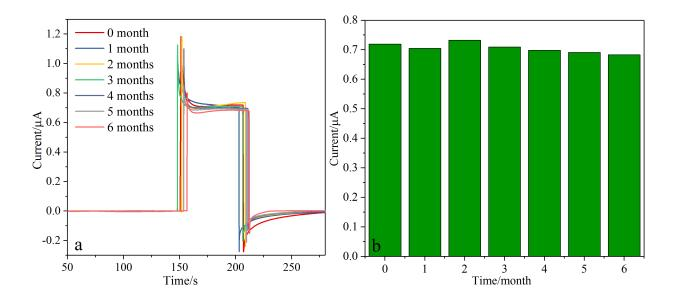
S8: Transient photocurrent curves (a) and photocurrents (b) in 0.1 M KCl aqueous solution recorded in continuous months.
