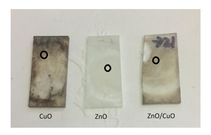
S2: Photos of CuO, ZnO, and ZnO/CuO NTs. The measuring area for SEM and UV-bis is circled.
