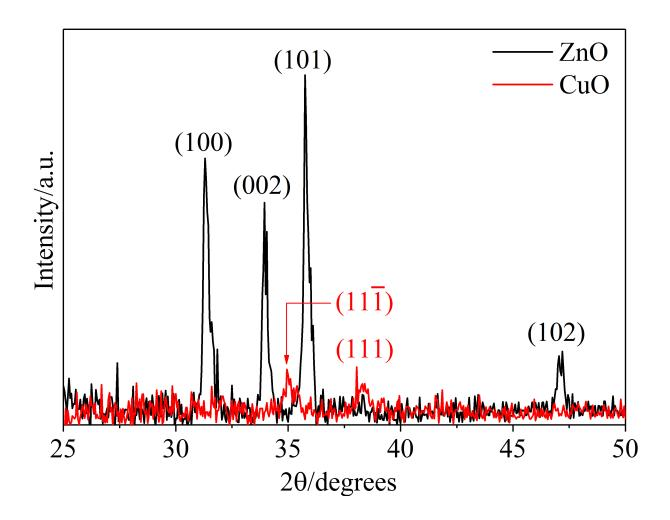
S4: High-resolution XRD spectra of ZnO nanowires in black and CuO nanorods in red.
