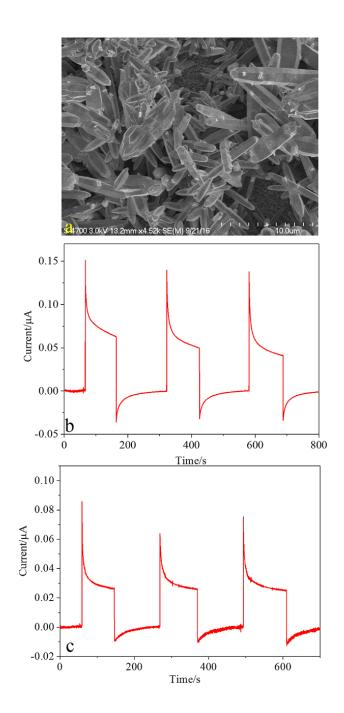
S11: a: SEM image of nontree structure of ZnO/CuO prepared without seeding process; b: transient photocurrent in 0.1 M KCl aqueous solution; and c:transient photocurrent in 0.1 M BuNF $_4$  in acetonitrile.
