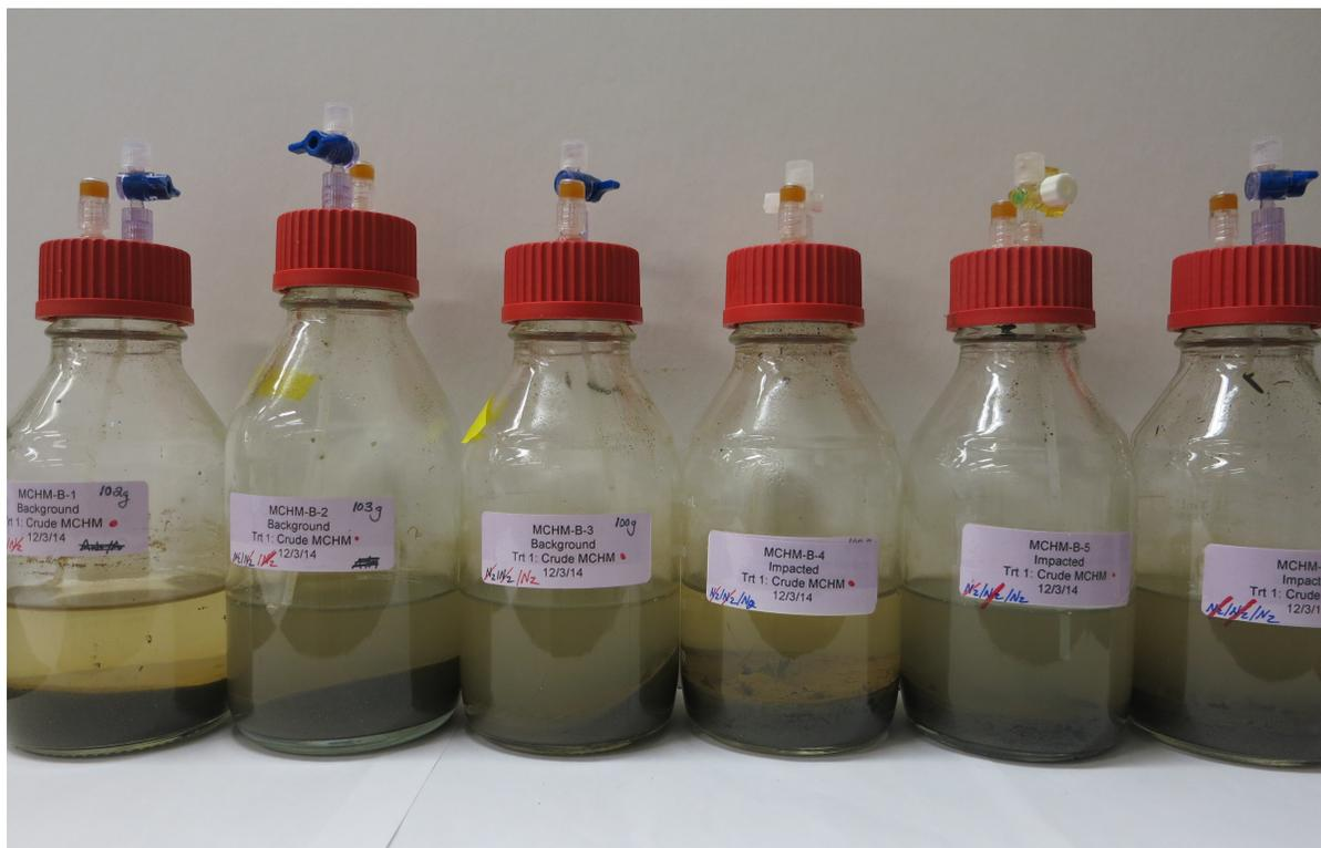
**Figure S1.** Photograph of biodegradation microcosms on day 25 amended with 1 mg/L crude MCHM. Left to right: Background sediment bottles B-1, B-2, and B-3; Impacted sediment bottles B-4, B-5, and B-6. Note the darker color in B-2, B-3, B-5, and B-6 which corresponds to the presence of Fe(II) from microbial iron reduction. Bottles B-1 and B-4 have a lighter color consistent with the lack of Fe(II) production observed due to air leakage (Table S3).
