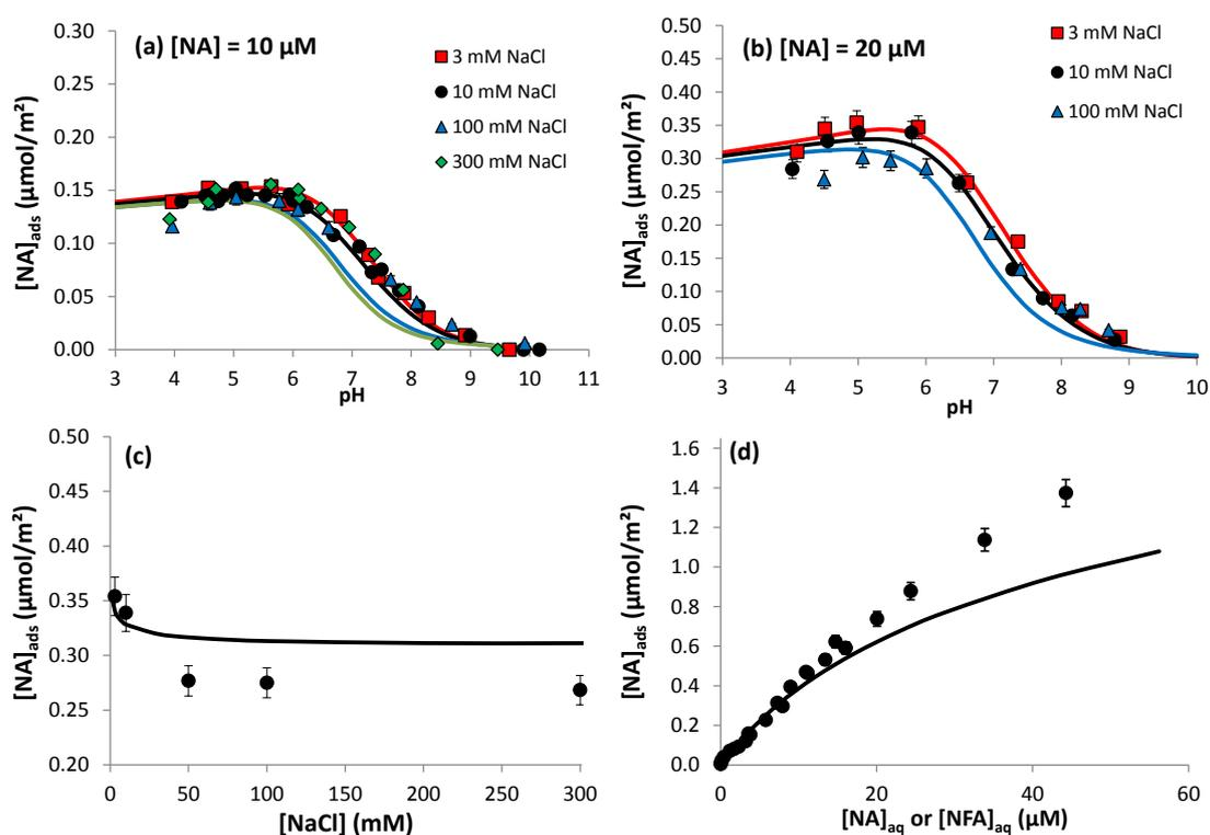
**Figure S2.** Modeling of single NA system, without considering NA dimer formation at goethite surface (preliminary model). (a) Adsorption of 10 μM NA to goethite (0.5 g/L) versus pH and [NaCl] (3-300 mM) (b) Adsorption of 20 μM NA to goethite (0.5 g/L) versus pH and [NaCl] (3-100 mM). (c) Adsorption of 20 μM NA to goethite (0.5 g/L) versus [NaCl] at pH 5. (d) NA-goethite adsorption isotherm at pH 6 in 10 mM NaCl.
