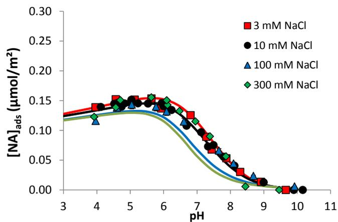
**Figure S3.** Modeling of single NA system, considering NA dimer formation at goethite surfaces (final model, see the main text for more details). Adsorption of 10  $\mu\text{M}$  NA to goethite (0.5 g/L) versus pH and  $[\text{NaCl}]$  (3-300 mM). Solid lines are modeling results (the same color as the corresponding symbol).
