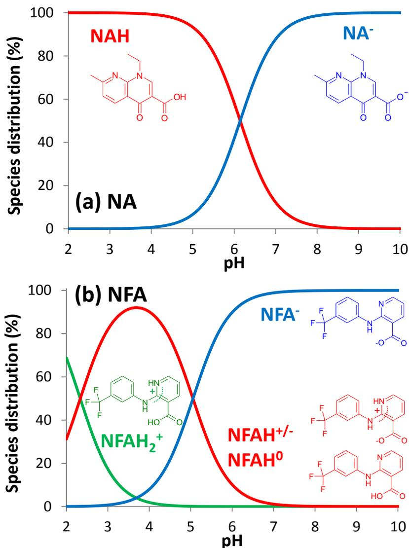
**Figure S1.** Distribution of (a) NA and (b) NFA at various pH values with molecular structures of different NA and NFA species. Ionic strength: 10 mM NaCl. pK<sub>a</sub>s of NA (pK<sub>a</sub>=6.19) and NFA (pK<sub>a,1</sub>=2.28 and pK<sub>a,2</sub>=5.10) at infinite dilution were obtained from conditional pK<sub>a</sub> values and the Davies equation.
