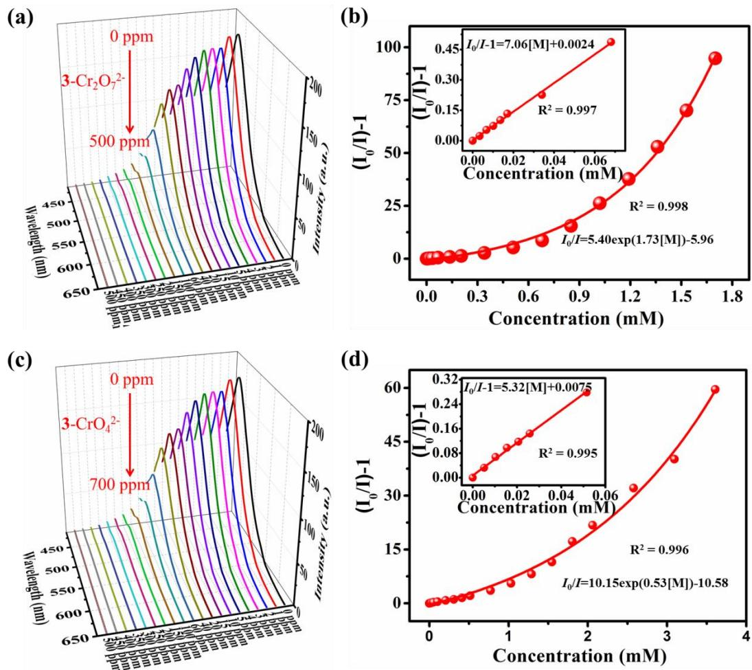
**Figure S19.** The emission spectra of **3** in aqueous solution with different concentrations of  $\text{Cr}_2\text{O}_7^{2-}$  (a) and  $\text{CrO}_4^{2-}$  (c) ions and the SV plots for  $\text{Cr}_2\text{O}_7^{2-}$  (b) and  $\text{CrO}_4^{2-}$  (d) ions.
