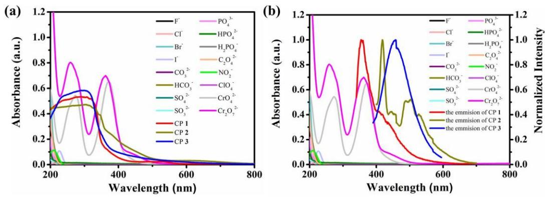
**Figure S22.** (a) The UV-vis absorption spectra of various anions in their aqueous solutions and the Solid state UV-vis absorption spectra of CPs **1-3**; (b) Spectral overlap between the UV-vis absorption spectra of spectra of various anions solutions and emission spectra of CPs **1-3** in water.
