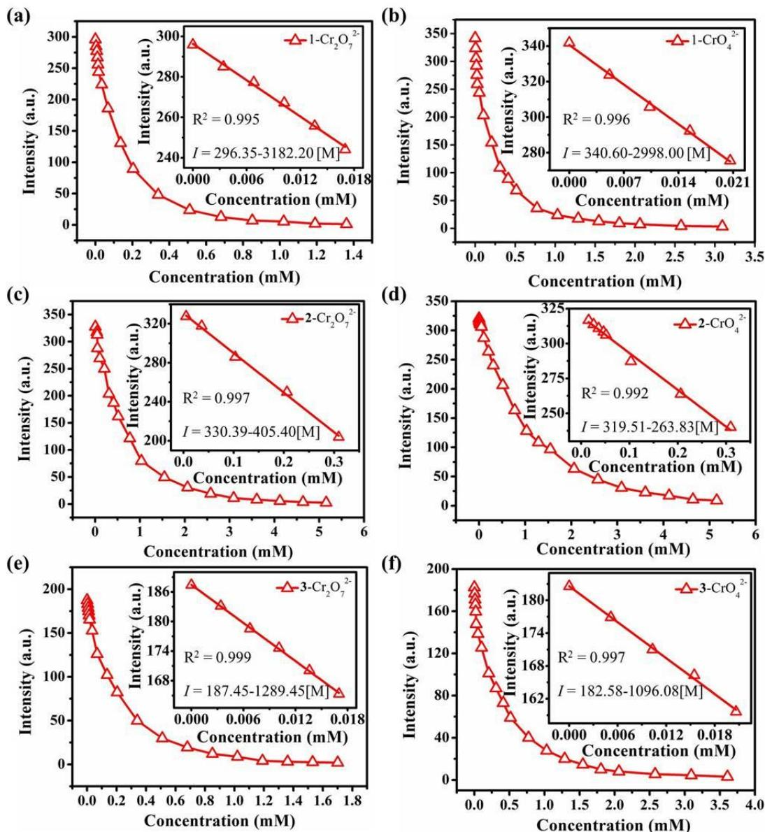
**Figure S21.** Changes of luminescent intensities with the maximum emission peaks of CPs **1** (a) and (b), **2** (c) and (d) and **3** (e) and (f), in aqueous solution with increasing concentrations of  $\text{Cr}_2\text{O}_7^{2-}$  and  $\text{CrO}_4^{2-}$  ions, and the linear relationships between intensities and the lower concentrations.
