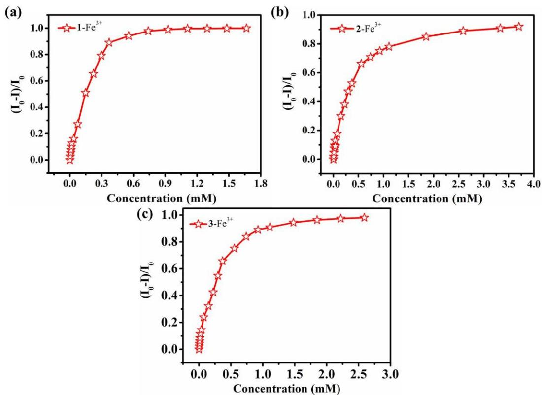
**Figure S12.** The quenching efficiency of CPs **1** (a), **2** (b) and **3** (c), in aqueous solution with different concentrations of  $\text{Fe}^{3+}$  ions.
