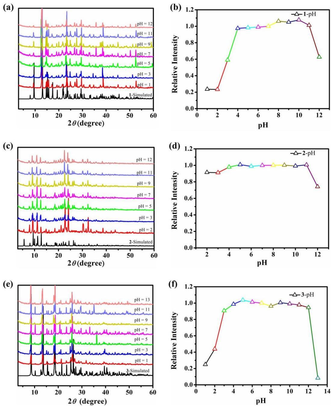
**Figure S9.** The PXRD patterns and the luminescent tests of CPs **1** (a) and (b), **2** (c) and (d), **3** (e) and (f) after being immersed in aqueous solution with different pH ranges, respectively.
