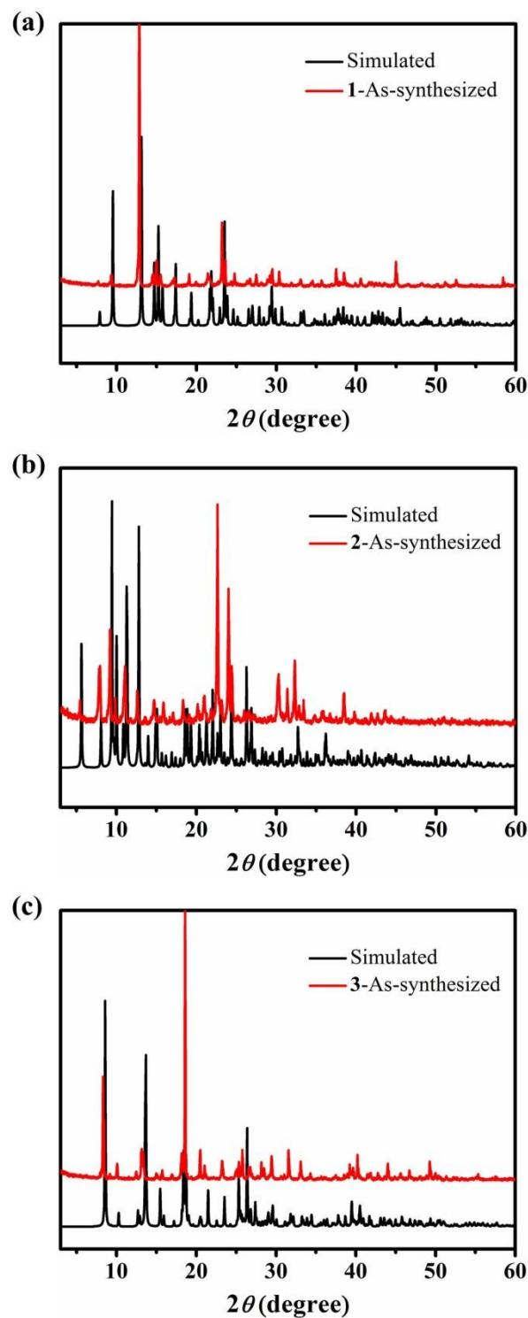
**Figure S6.** PXRD patterns of the synthesized samples and simulated patterns from single crystal data of CPs **1** (a), **2** (b) and **3** (c).
