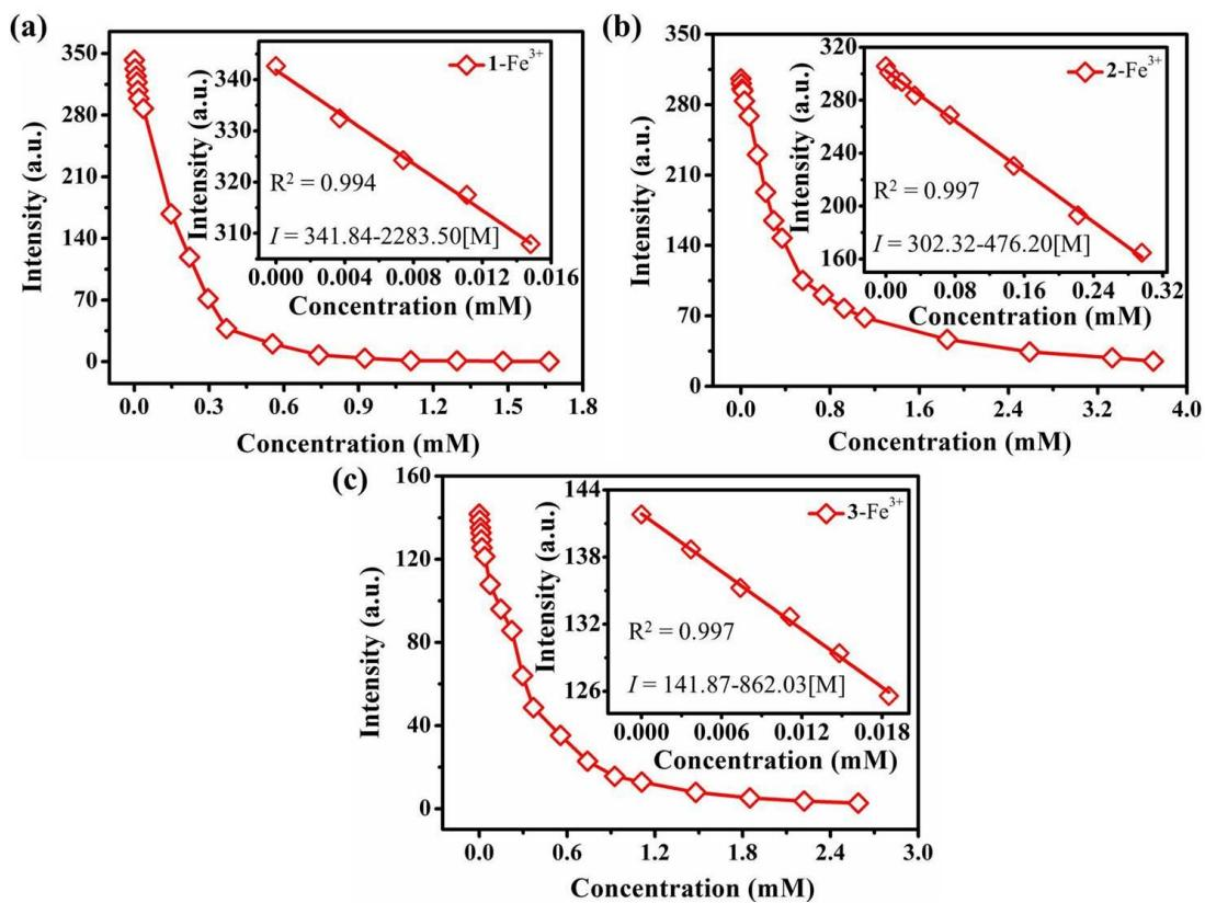
**Figure S13.** Changes of luminescent intensities with the maximum emission peaks of CPs **1** (a), **2** (b) and **3** (c), in aqueous solution with increasing concentrations of  $\text{Fe}^{3+}$  ions., insets display the linear relationships between intensities and the lower concentrations.
