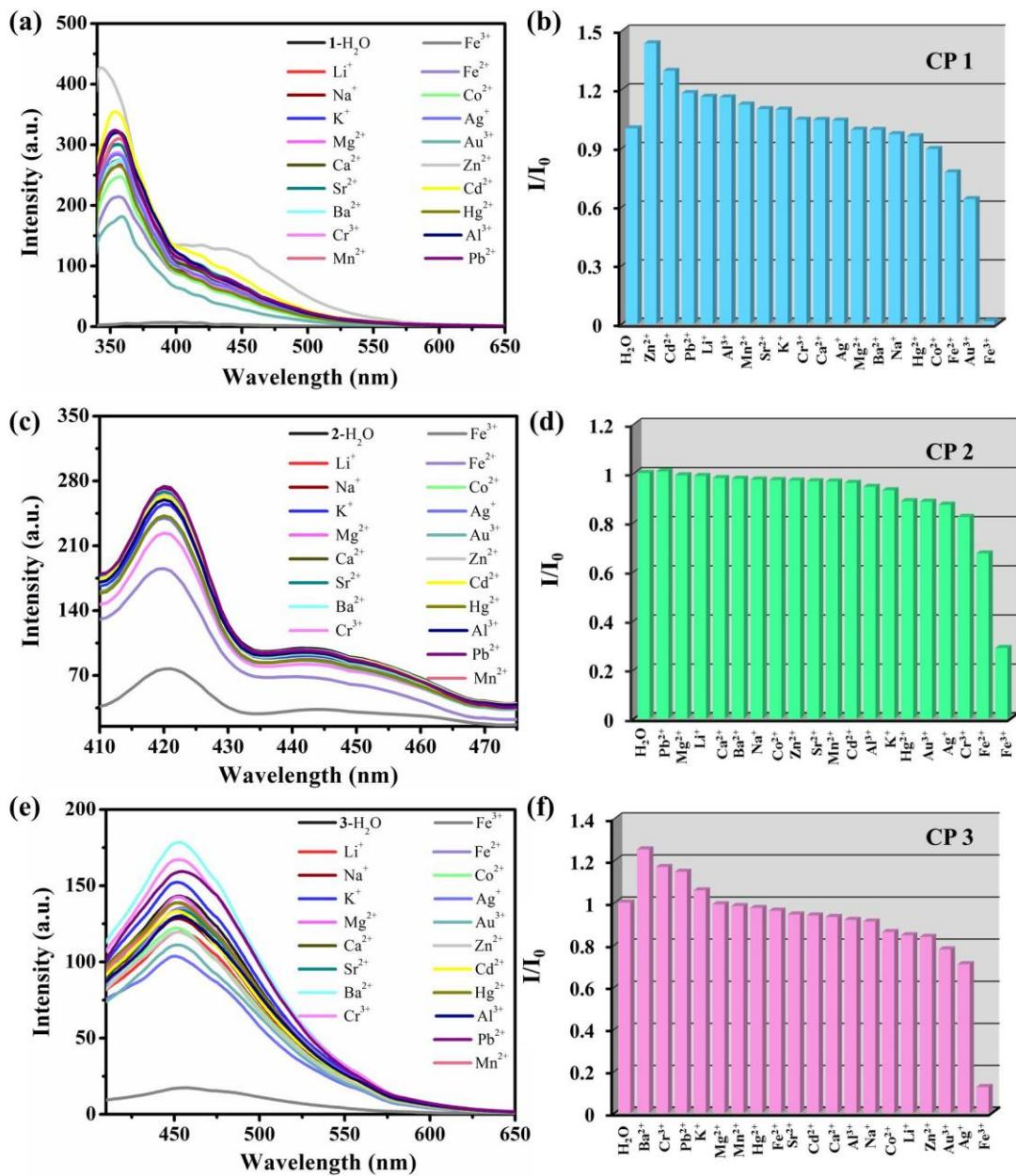
**Figure S11.** Suspension-state luminescent spectra of CPs **1** (a), **2** (c) and **3** (e), and the maximum emission intensities of CPs **1** (b), **2** (d) and **3** (f) with different metal cations ( $1\times 10^{-3}\text{ M}$ ).
