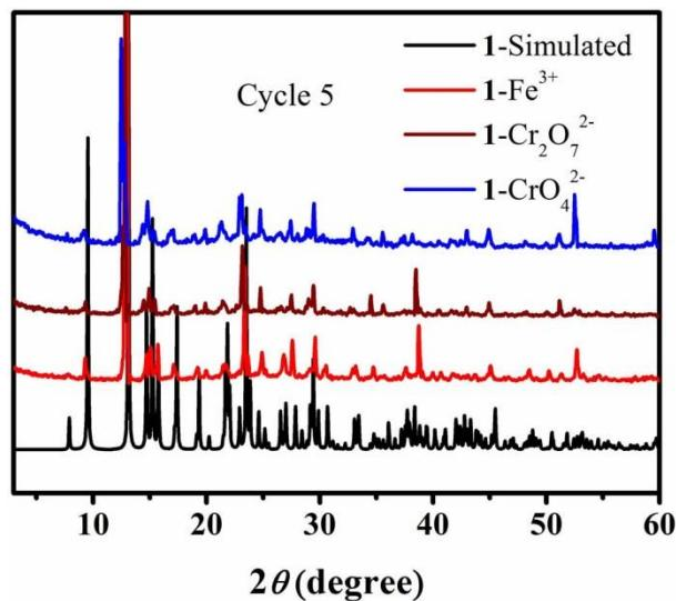
**Figure S14.** The PXRD patterns of CPs **1** after five cycles tests.
