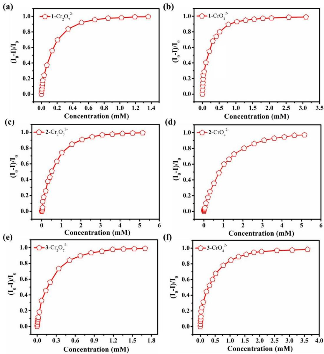
**Figure S20.** The quenching efficiency of CPs **1** (a) and (b), **2** (c) and (d) and **3** (e) and (f), in aqueous solution with different concentrations of  $\text{Cr}_2\text{O}_7^{2-}$  and  $\text{CrO}_4^{2-}$  ions.
