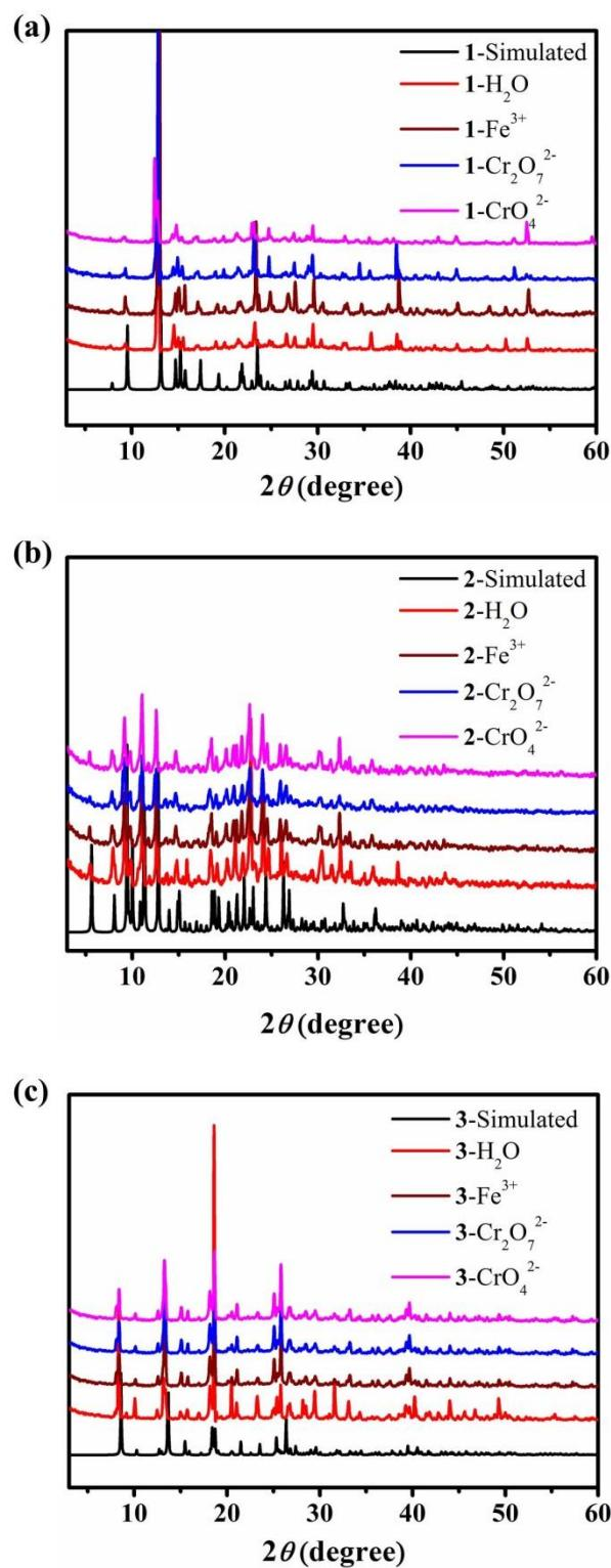
**Figure S15.** The PXRD patterns of CPs **1** (a), **2** (b) and **3** (c) after sensing for Fe<sup>3+</sup>, Cr<sub>2</sub>O<sub>7</sub><sup>2-</sup> and CrO<sub>4</sub><sup>2-</sup> ions in aqueous solution.
