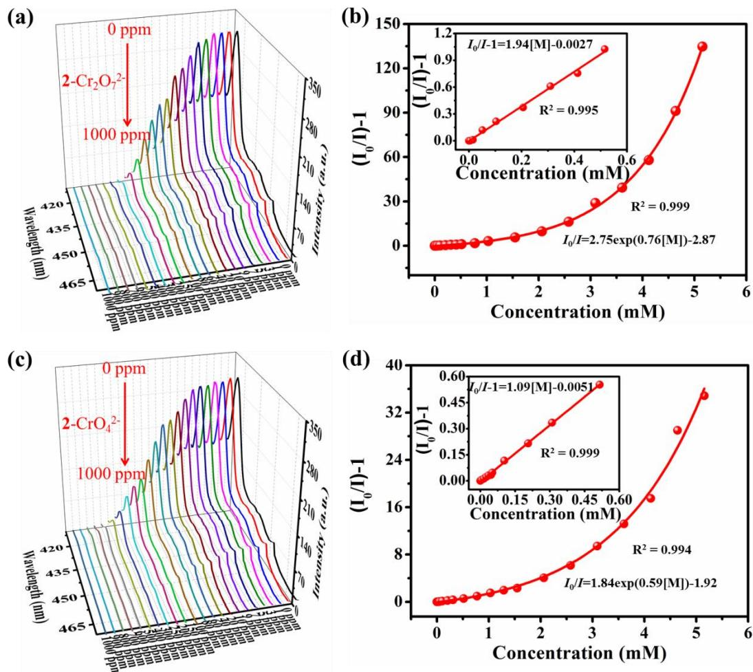
**Figure S18.** The emission spectra of **2** in aqueous solution with different concentrations of  $\text{Cr}_2\text{O}_7^{2-}$  (a) and  $\text{CrO}_4^{2-}$  (c) ions and the SV plots for  $\text{Cr}_2\text{O}_7^{2-}$  (b) and  $\text{CrO}_4^{2-}$  (d) ions.
