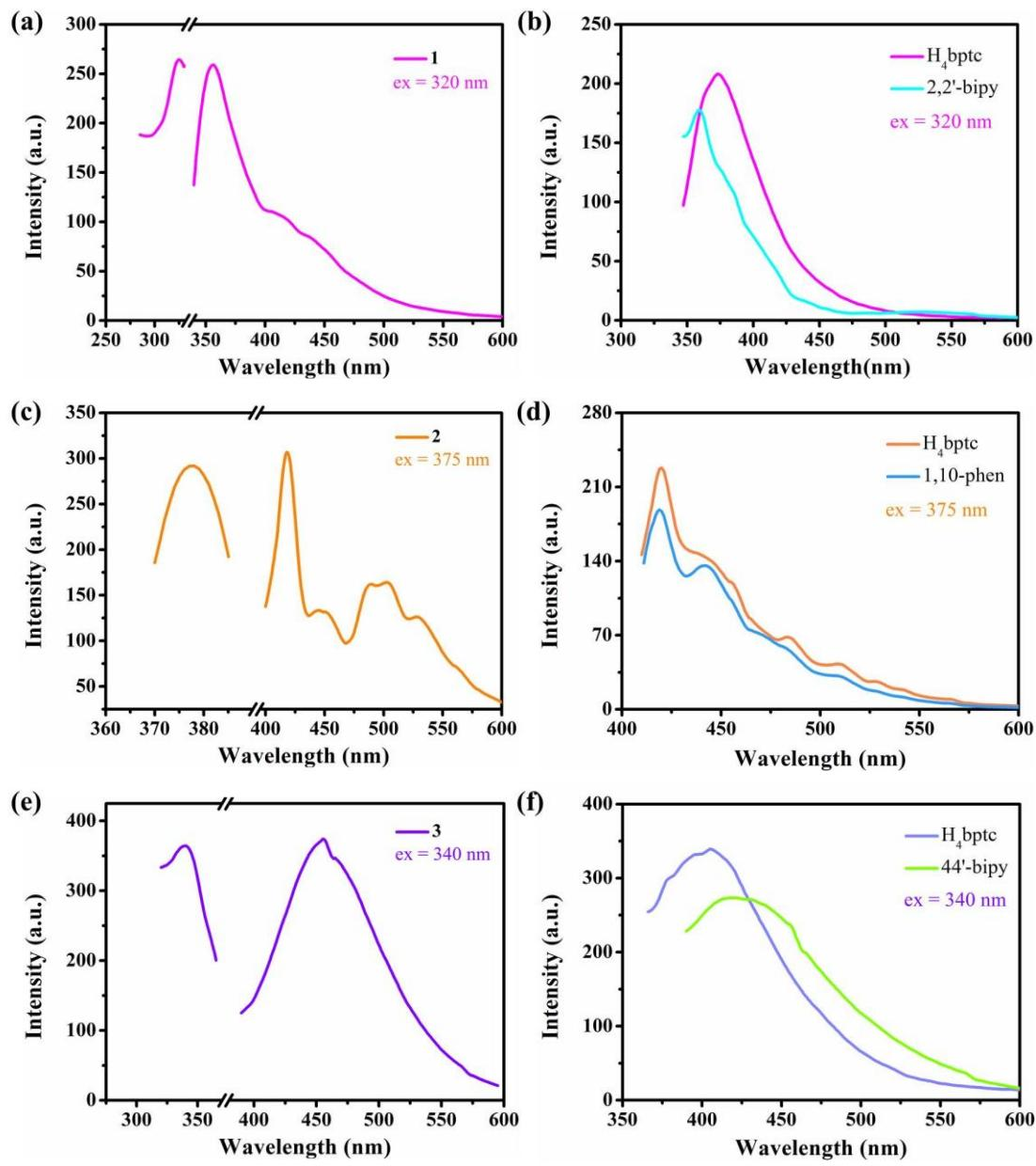
**Figure S8.** The room temperature solid-state excitation and emission spectra of CPs **1** (a), **2** (c), **3** (e), and the emission spectra of free ligands in CPs **1** (b), **2** (d), **3** (f), respectively.
