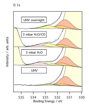
O 1s core- level NAP-XPS spectra recorded at UHV, under exposure to 3 mbar  $H_2O$ , under exposure to 3mbar  $H_2O/CO$  and at UHV the following day. The O 1s spectra highlight the high binding energy shoulder shown in Figure 4 of the main manuscript for clarity.
