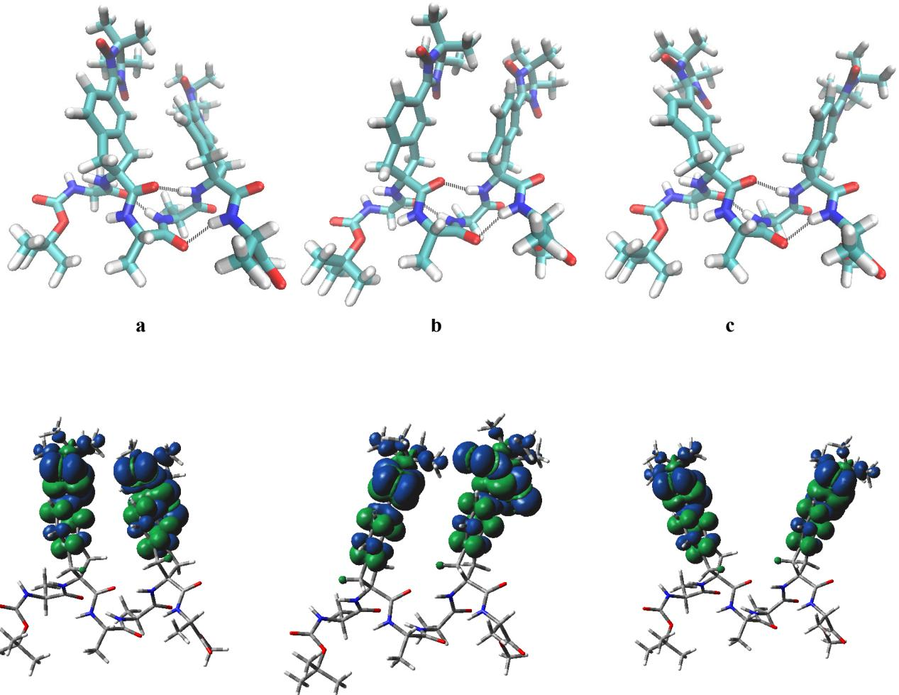
**Figure S4.** Top: optimized 3D-structures for the bis-(R)-Aic(NN) hexapeptide with the intramolecular H-bonds highlighted (distance cutoff 3.1 Å, angle cut-off 20°). Considering the Gibbs free energy: **c** is the most stable structure, **a** is 0.3 kcal/mol higher, and **b** is 2.2 kcal/mol higher. Bottom: spin densities are highlighted (in green and blue, respectively, according to the phase).
