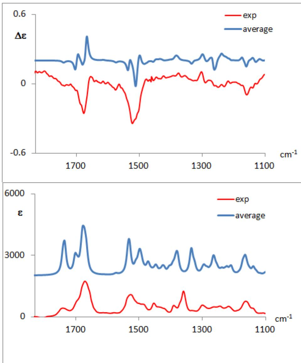
**Figure S3.** Experimental and calculated IR absorption and VCD spectra for the bis-(R)-Aic(NN) hexapeptide. The calculated spectra correspond to a weighted average of the two conformers **a** and **c** (37%, 63%). For a better comparison, the calculated wavenumbers have been scaled by 0.97.
