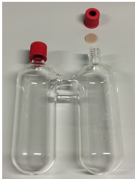
Figure S3. Large two-chamber reactor. Inner volume = 400 mL. Invented by the Skrydstrup group. 2
