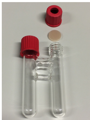
Figure S2. Small two-chamber reactor. Inner volume = 20 mL. Invented by the Skrydstrup group. 2
