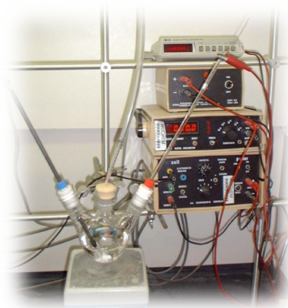
Figure 1 Anodic Cyclization Reaction Apparatus
