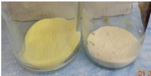
Figure S7. Example of color change of dry solid containing UiO-66(NH 2 ) precursors on silica A (intense yellow, left) and after solid-state synthesis for 2 hours at 120 °C in the oven (pale yellow, right).
