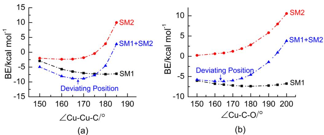
**Figure S3.**  $\omega$ B97XD-calculated potential energy surfaces for CO interactions with (a) SM1 and (b) SM2 models.
