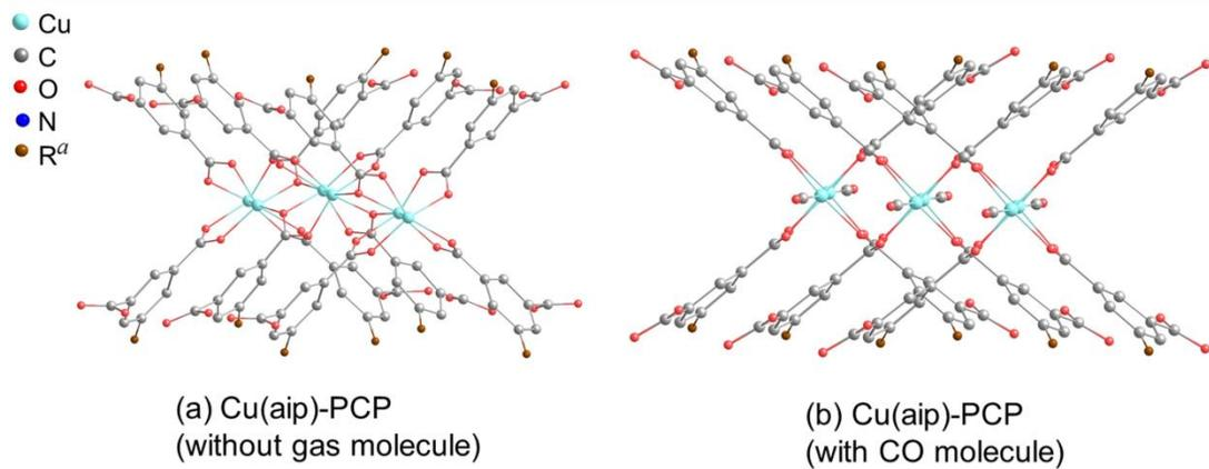
**Figure S1.** Another side view of structures of Cu(aip)-PCP (a) without gas molecule and (b) with adsorbed CO molecules.
