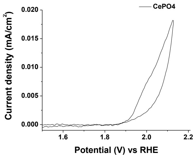
**Figure S5.** Cyclic voltammetry for OER using CePO<sub>4</sub> thin film.
