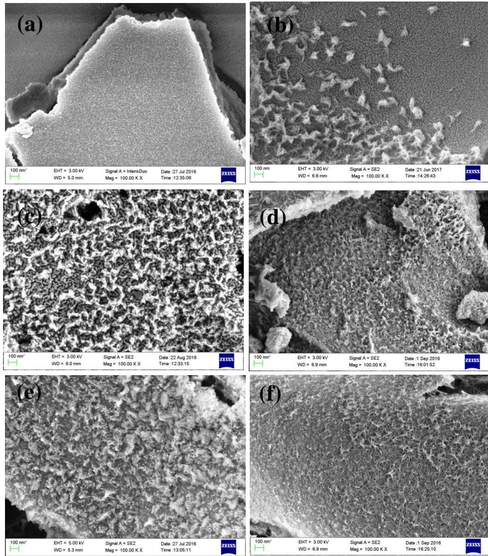
**Figure S2.** FESEM images of FePH films formed with different amount of cerium acetate **(a)** FePH, **(b)** FeCePH1, **(c)** FeCePH2, **(d)** FeCePH3, **(e)** FeCePH4 and **(f)** FeCePH5. Scale bar= 100 nm.
