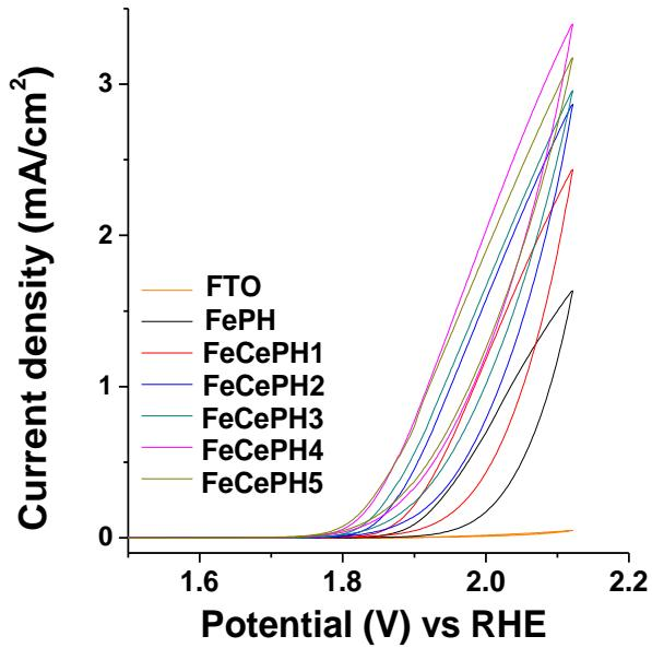
**Figure S4.** CVs for electrochemical OER using FePH and FeCePHX film catalysts at scan rate = 5 mV/s
