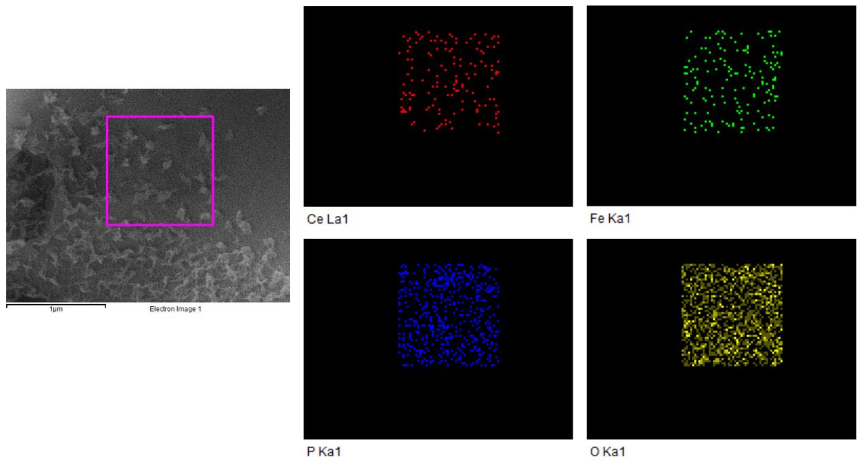
**Figure S3.** FESEM images of FeCePH1 with EDXS area color mapping.
