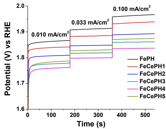
**Figure S6.** Plots of potential versus time for electrolysis carried out at 0.01, 0.033 and 0.1 mA/cm<sup>2</sup> current densities for 3 min each, using the different thin film catalysts.
