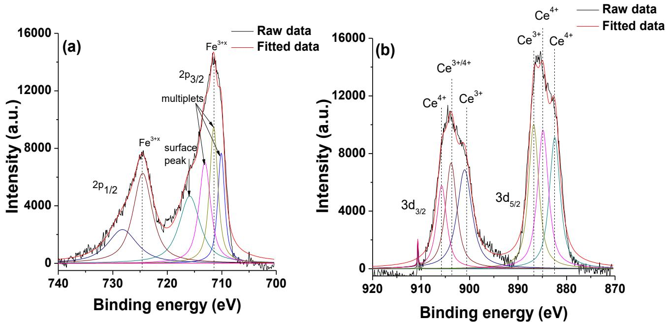
**Figure S8.** XPS spectra of (a) Fe ( $2p_{1/2}$ ,  $2p_{3/2}$ ) and (b) Ce ( $3d_{3/2}$ ,  $3d_{5/2}$ ) of FeCePH4 film after electrolysis at 1.9 V vs RHE for 3 h.
