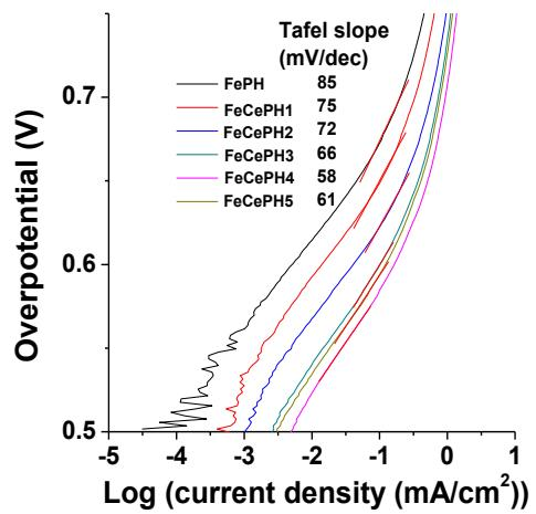
**Figure S7.** Tafel plots derived from the anodic current density of CV.
