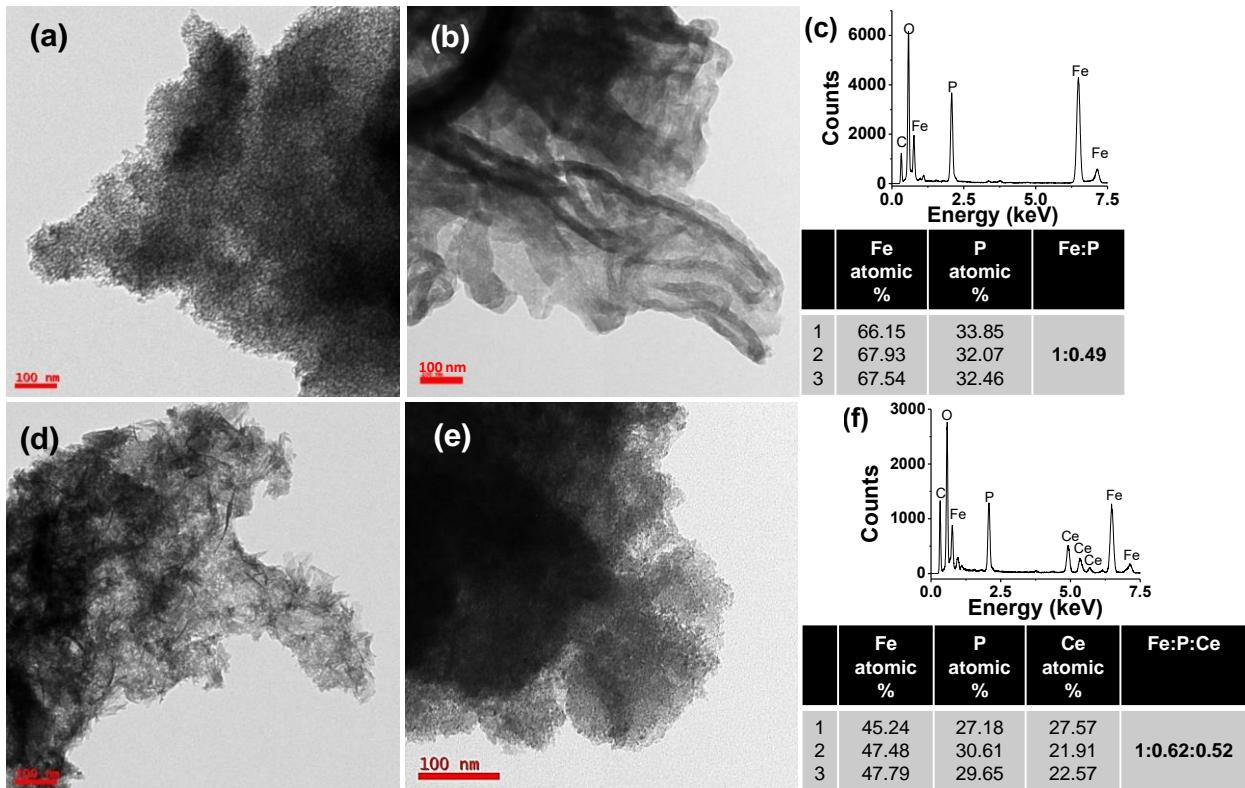
**Figure S9.** TEM image (a) before and (b) after catalysis, and (c) EDX spectrum and analysis after catalysis, of FePH film; (d, e, f) are corresponding figures for FeCePH4.
