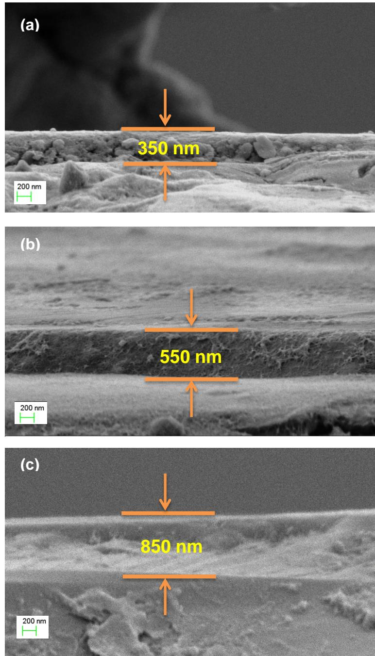
**Figure S1.** Thickness of the film from FESEM analysis; (a) FePH, (b) FeCePH2 and (c) FeCePH4; electrocatalyst films coated on closely placed substrate plates were sectioned by taking the substrates apart, and the cross-section imaged.
