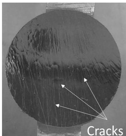
**Figure S6.** Image of actuated silver electrode.
