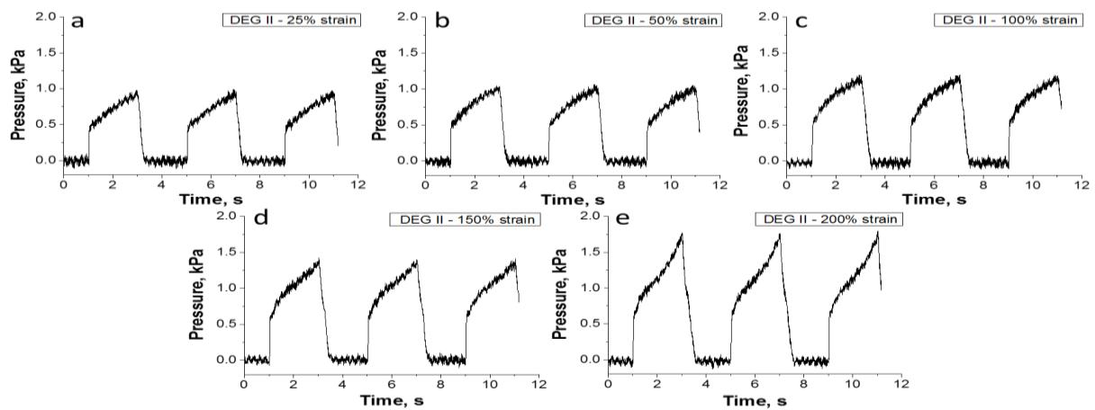
**Figure S11.** Inside air chamber pressure during harvesting cycles of DEG II.
