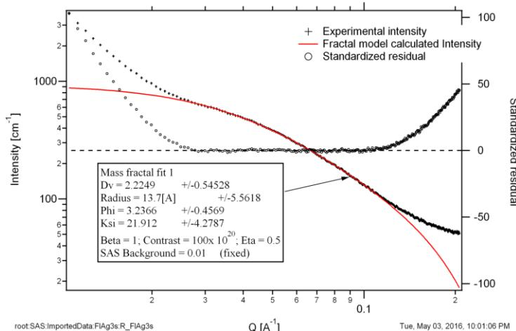
**Figure S3.** Fitting plot of fractal model.
