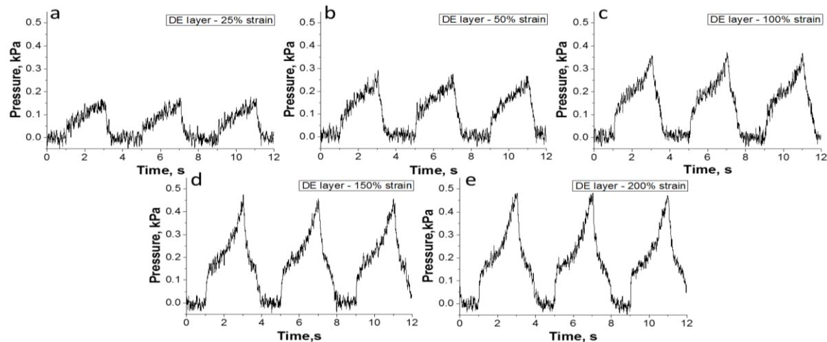
**Figure S9.** Inside air chamber pressure during harvesting cycles of a single DE layer.
