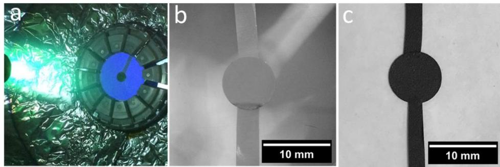
**Figure S5.** a) Image during deposition of silver electrode; b) silver electrode deposited on DE used in actuation measurements; c) PDMS-Cb electrode attached on DE used in actuation measurements.
