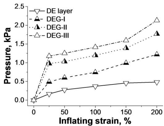
**Figure S8.** Pressure needed to inflate the DEG, depending on the number of dielectric layers.
