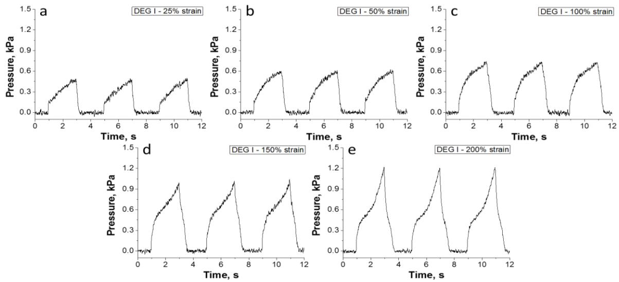
**Figure S10.** Inside air chamber pressure during harvesting cycles of DEG I.
