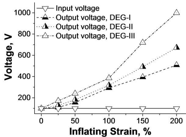
**Figure S13.** Measured output voltage and inflating pressure as a function of inflating strain,
