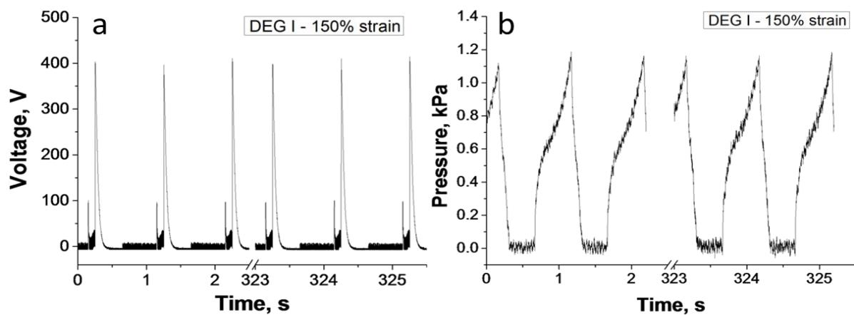
**Figure S18.** Variation of harvested voltage (a) and air chamber pressure (b) depending on the number of cycles.
