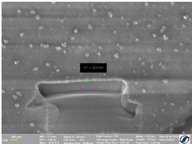
**Figure S1.** FIB-SEM image of silver electrode deposited on silicone dielectric.
