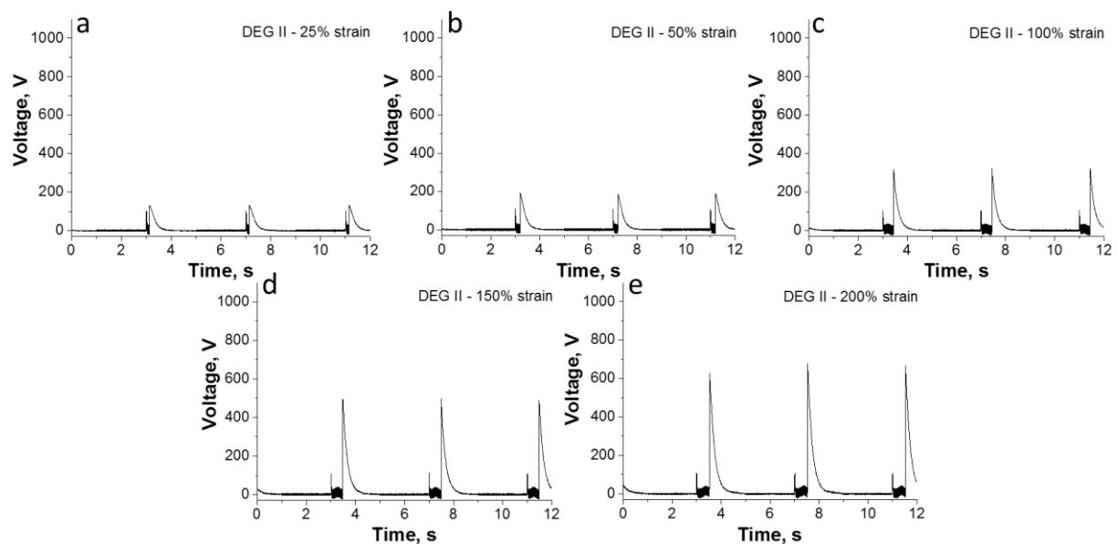
**Figure S15.** Harvested voltage of DEG II.
