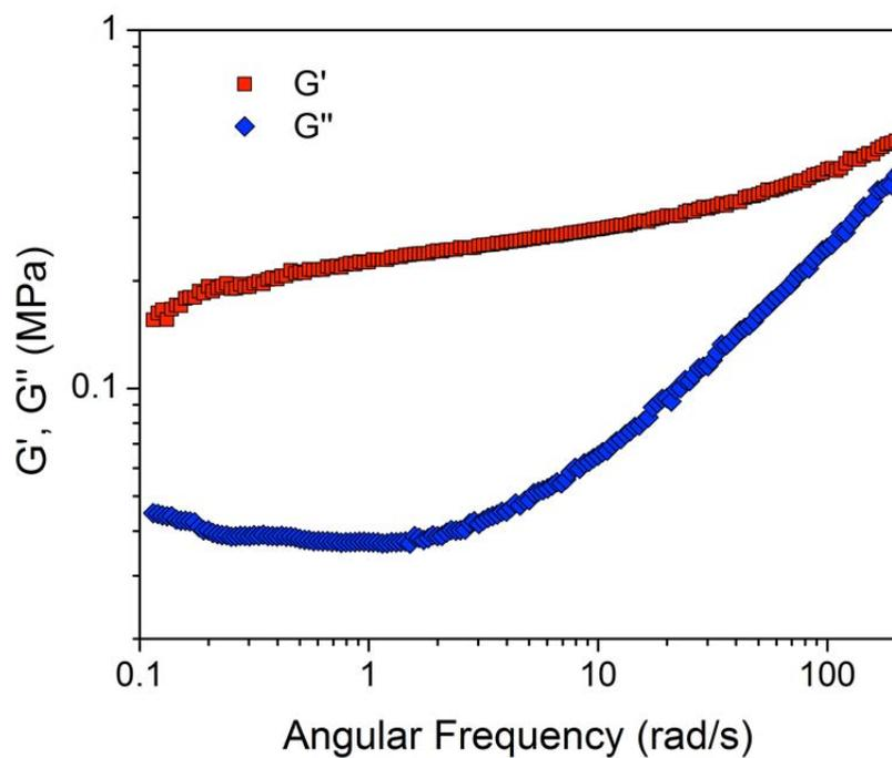
**Figure S6.** Dynamic mechanical analysis of hPNbN ( $M_n = 247$  kg/mol,  $D = 1.14$ ) at 160 °C. The minimum in  $G''$  occurs at  $\omega = 1.14$  rad/s, corresponding to  $G' = 0.22$  MPa.
