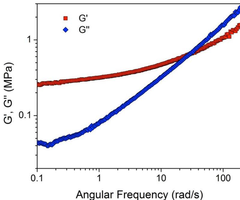
**Figure S5.** Dynamic mechanical analysis of hPCyN ( $M_n = 252$  kg/mol,  $\mathcal{D} = 1.23$ ) at 120 °C. The minimum in  $G''$  occurs at  $\omega = 0.15$  rad/s, corresponding to  $G' = 0.27$  MPa.
