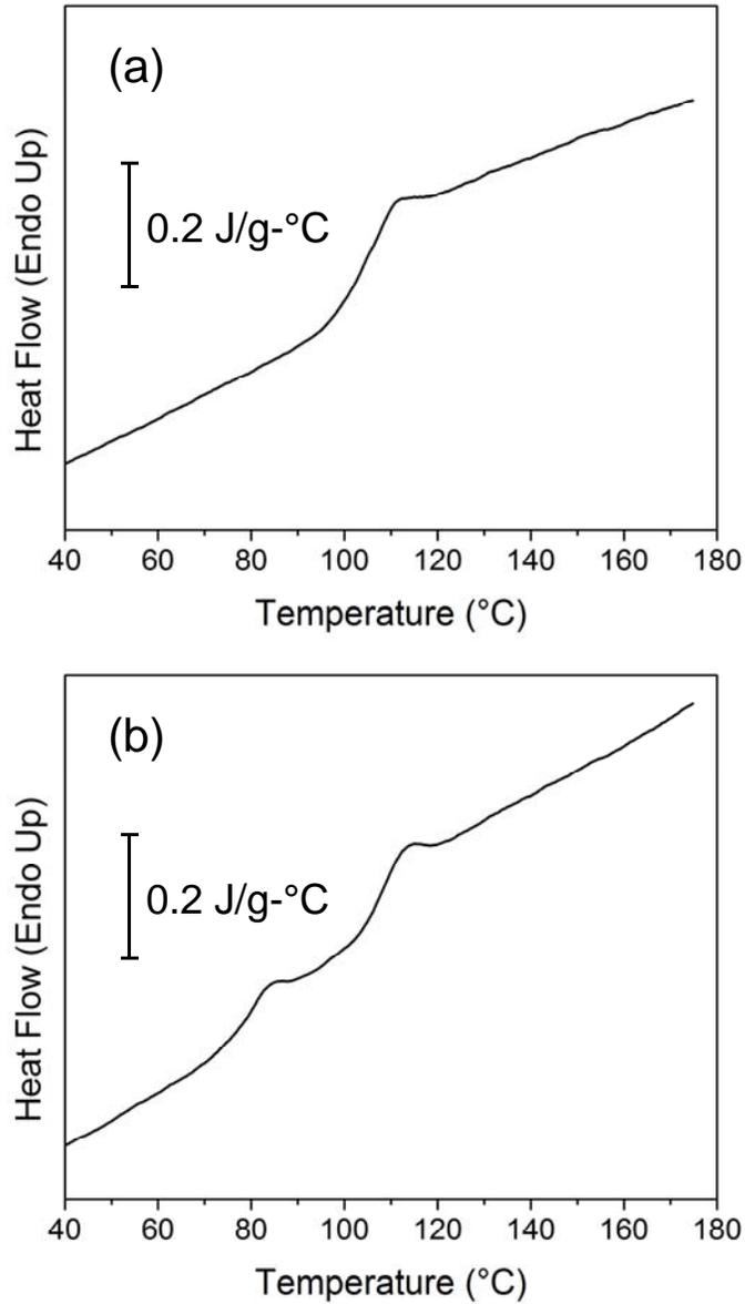
**Figure S10.** DSC traces of (a) 122 kg/mol hPCyN and 123 kg/mol hPNbN with  $\phi_{\text{hPCyN}} = 0.50$  (single-phase), and (b) 122 kg/mol hPCyN and 158 kg/mol hPNbN with  $\phi_{\text{hPCyN}} = 0.52$  (phase-separated).
