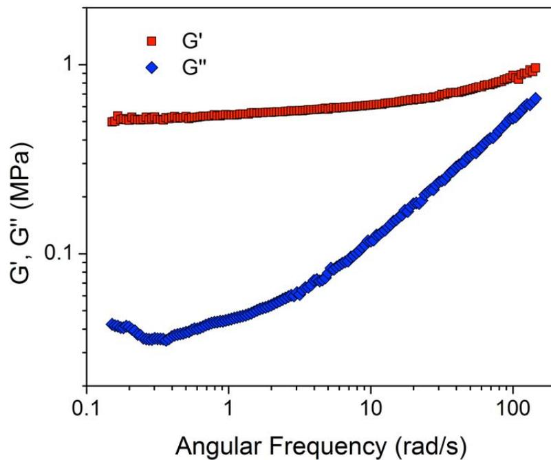
**Figure S7.** Dynamic mechanical analysis of hPPhN ( $M_n = 278$  kg/mol,  $D = 1.09$ ) at 100 °C. The minimum in  $G''$  occurs at  $\omega = 0.36$  rad/s, corresponding to  $G' = 0.52$  MPa.
