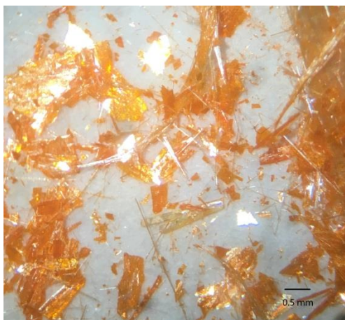
Figure S1. Photograph of the three types of crystals obtained: bright orange platelets ( ((\text{C}_6\text{H}_5\text{CH}_2\text{NH}_3)_2\text{PbI}_4) ), colorless needles (an unidentified phase), and nearly transparent, light yellow bar-shaped crystals ( ((\text{C}_6\text{H}_5\text{CH}_2\text{NH}_3)_4\text{Pb}_5\text{I}_{14} \cdot 2\text{H}_2\text{O}) ).
