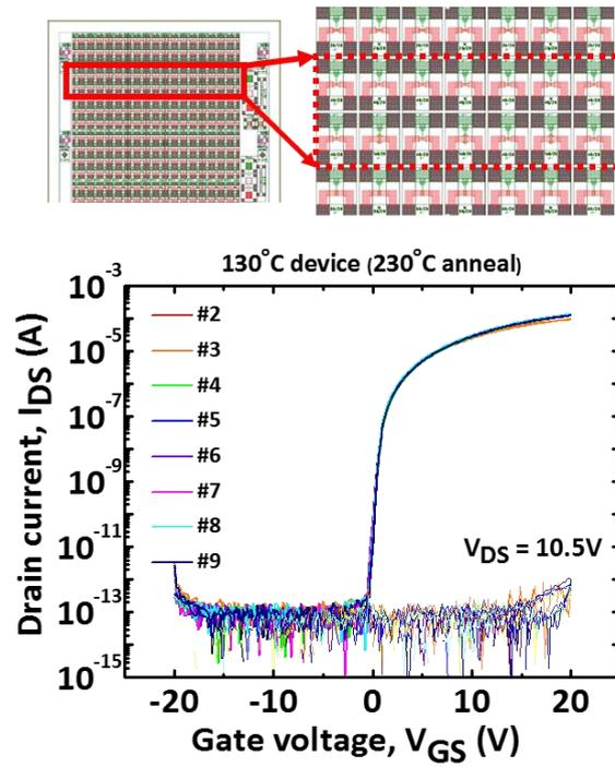
This supporting information shows typical examples of device-to-device uniformity in transfer characteristics of the TFTs using the IGZO channel deposited at 130 °C and annealed at 230 °C, as shown in Figure S3. The number of evaluated devices were 9 in this case.
