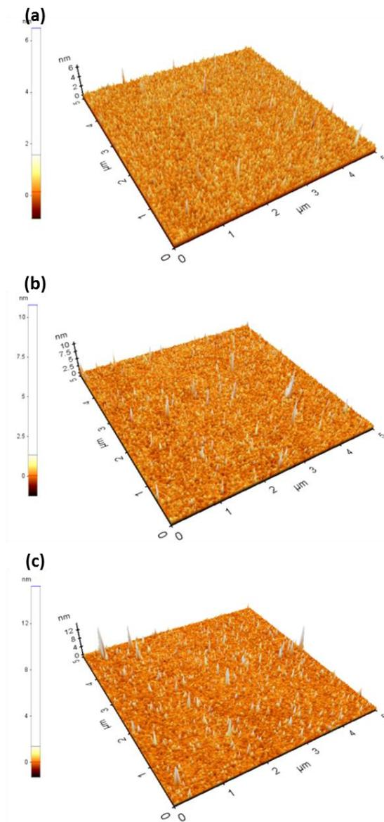
This supporting information exhibits the atomic force microscope (AFM) images of the IGZO films deposited at different ALD temperatures of 130, 150, and 170 °C in a 5×5 μm scan area. The root-mean square surface roughness ( $R_q$ ) of the IGZO films showed an increasing trend as the ALD temperatures increased, in which the  $R_q$  values were estimated to be approximately 0.30, 0.34, and 0.46 nm for the IGZO films deposited at 130, 150, and 170 °C, respectively, as shown in Figure S1.
