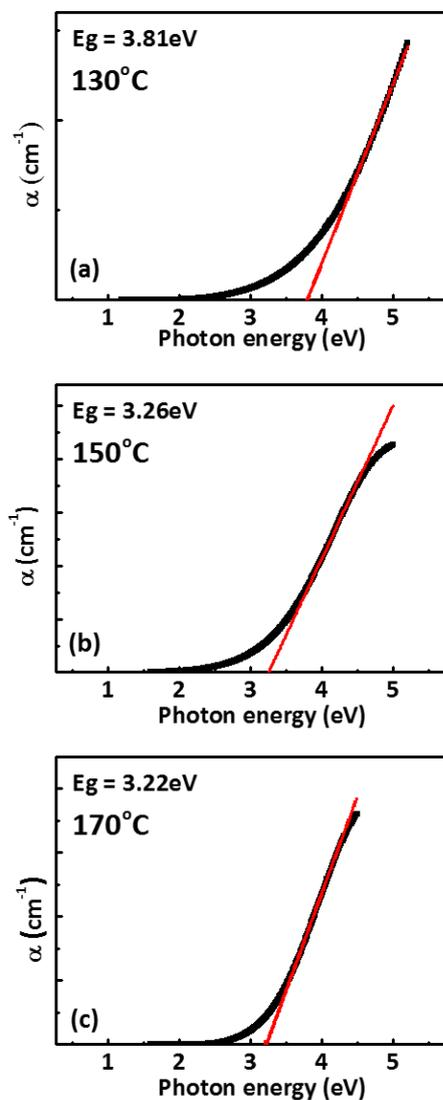
This supporting information shows the curve fittings of the absorption coefficient as a function of the photon energy measured by spectroscopic ellipsometer (SE J. A. Woolam Co.) analyzer. The calculated optical band gaps of the IGZO films appeared to be 3.81, 3.26, and 3.21 eV when the ALD temperatures were controlled to be 130, 150, and 170 °C, respectively, as shown in Figure S2.
