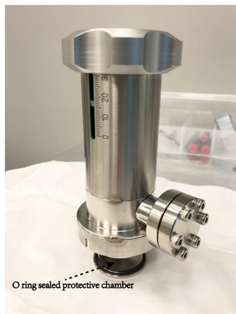
Figure S3. Picture of the vacuum vessel for XPS sample transfer.
