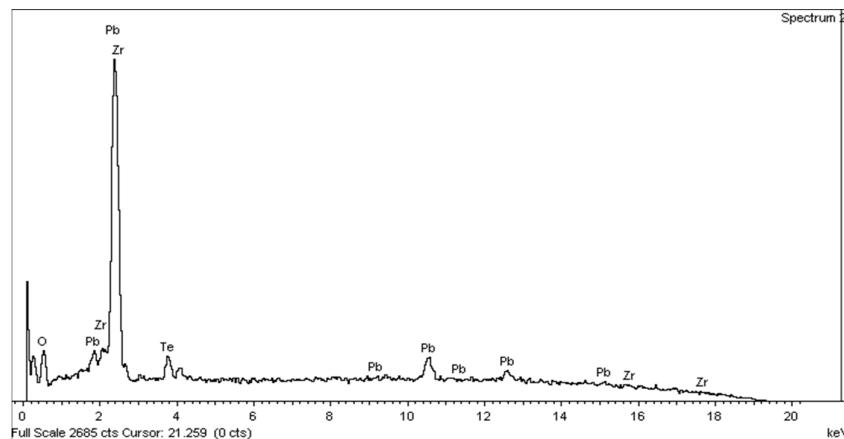
Figure S3. Energy-Dispersive Spectrometry (EDS) for  $\text{Pb}_9\text{Te}_2\text{O}_{13}(\text{OH})(\text{NO}_3)_3$ .
