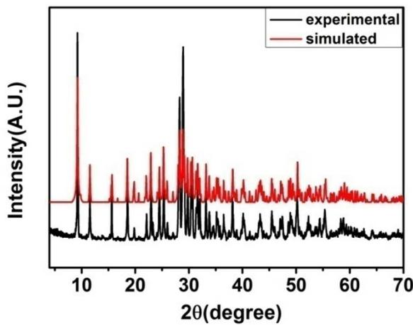
Figure S2. Experimented powder X-ray diffraction patterns (black line) of  $\text{Pb}_9\text{Te}_2\text{O}_{13}(\text{OH})(\text{NO}_3)_3$  compared to the calculated from the crystal data (red line).
