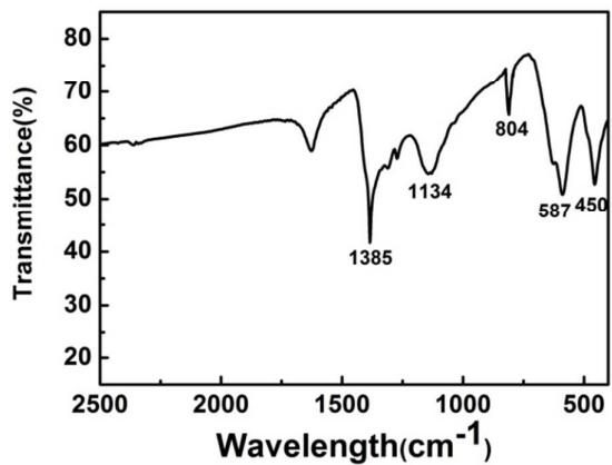
Figure S6. Infrared spectra of  $\text{Pb}_9\text{Te}_2\text{O}_{13}(\text{OH})(\text{NO}_3)_3$ .
