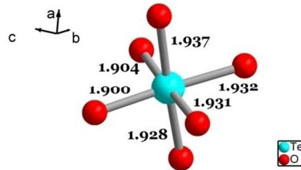
Figure S4. The coordinate environments of the  $\text{Te}^{6+}$  cations of  $\text{Pb}_9\text{Te}_2\text{O}_{13}(\text{OH})(\text{NO}_3)_3$ .
