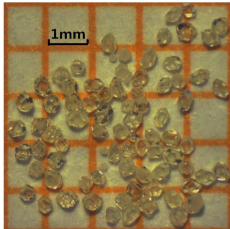
Figure S1. The morphology for  $\text{Pb}_9\text{Te}_2\text{O}_{13}(\text{OH})(\text{NO}_3)_3$ .
