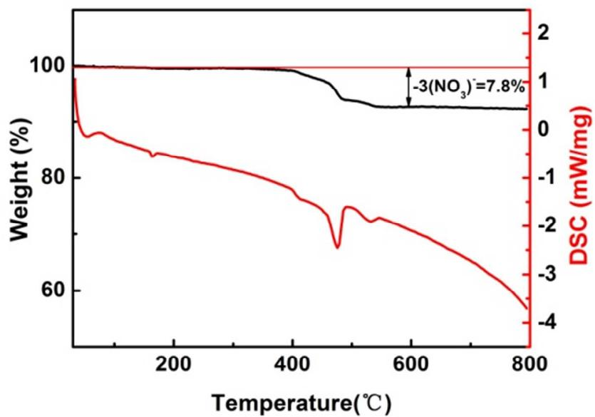
Figure S7. The TGA and DSC curves for  $\text{Pb}_9\text{Te}_2\text{O}_{13}(\text{OH})(\text{NO}_3)_3$  in 30-800°C range.
