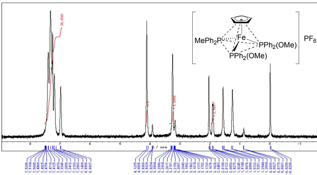
**Figure S24-1.**  $^1\text{H}$  NMR Spectrum of  $[\text{CpFe}(\text{PPh}_2\text{Me})\{\text{PPh}_2(\text{OMe})\}_2]\text{PF}_6$  in  $\text{CDCl}_3$  at 293 K.
