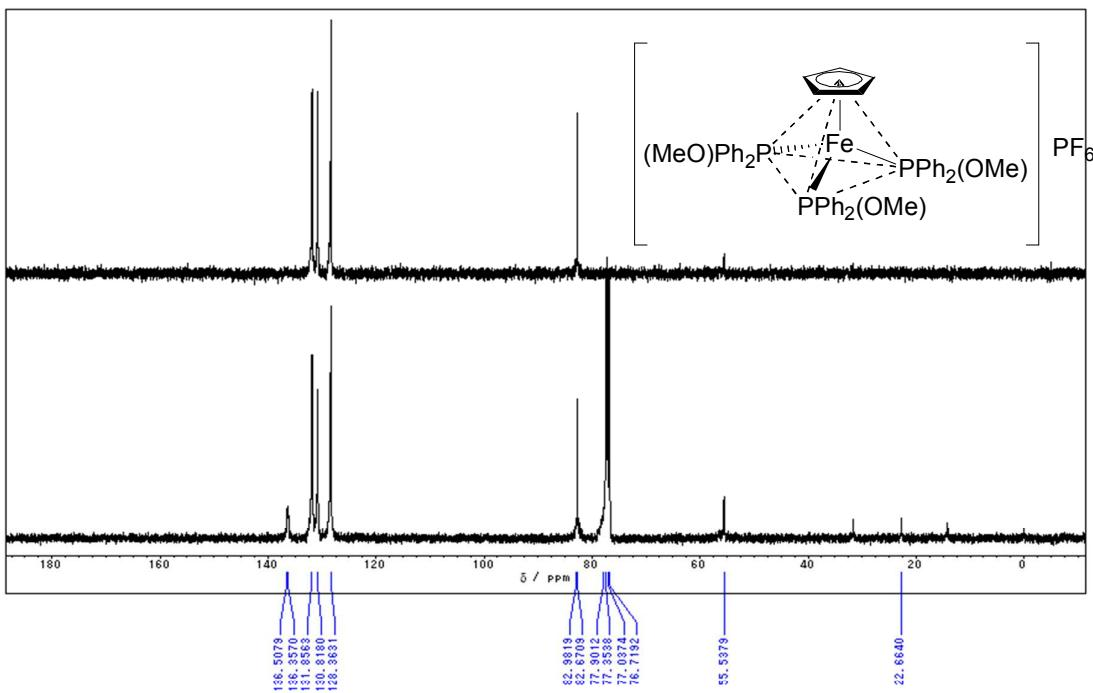
**Figure S26-2.**  $^{13}\text{C}$  NMR Spectra of  $[\text{CpFe}\{\text{PPh}_2(\text{OMe})\}_3]\text{PF}_6$  in  $\text{CDCl}_3$  at 293 K (top: DEPT135, bottom: decoupling).
