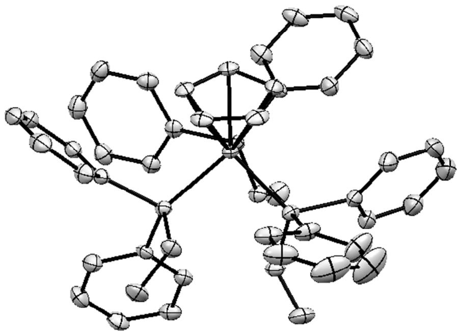
**Figure S26-4.** ORTEP drawing of  $[\text{CpFe}\{\text{PPh}_2(\text{OMe})\}_3]\text{PF}_6$ . Hydrogen atoms, hexafluorophosphate anion,  $\text{CH}_2\text{Cl}_2$  molecule are omitted for clarity.
