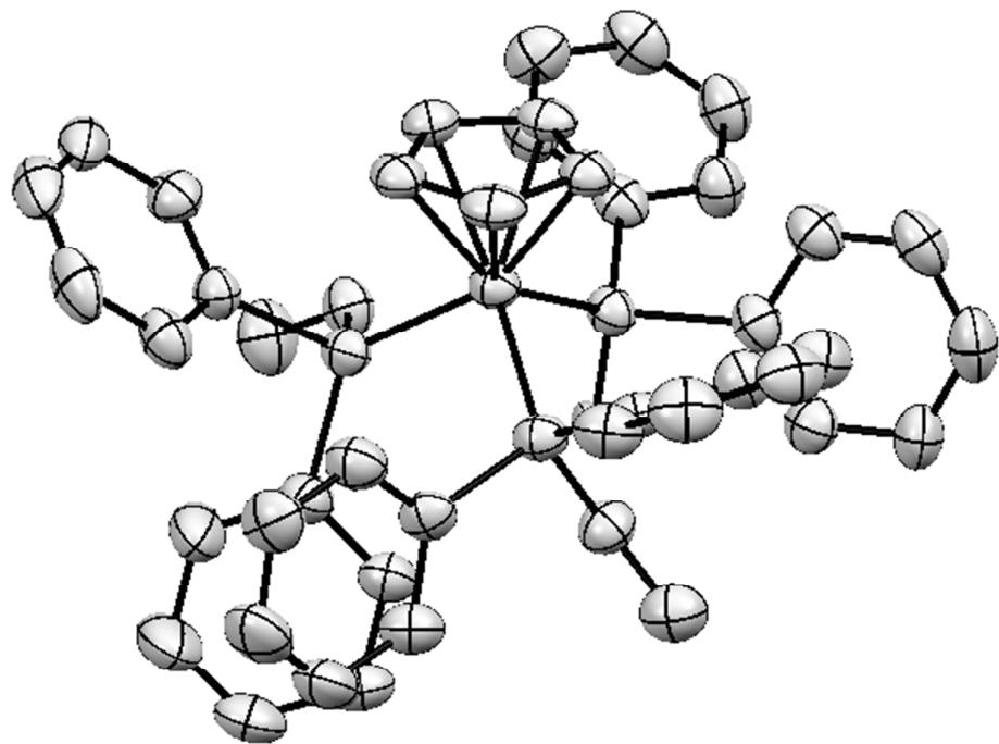
**Figure S24-3.** ORTEP drawing of  $[\text{CpFe}(\text{PPh}_2\text{Me})\{\text{PPh}_2(\text{OMe})\}_2]\text{PF}_6 \cdot 2\text{CH}_2\text{Cl}_2$ . Hydrogen atoms, hexafluorophosphate anion and  $\text{CH}_2\text{Cl}_2$  molecules are omitted for clarity.
