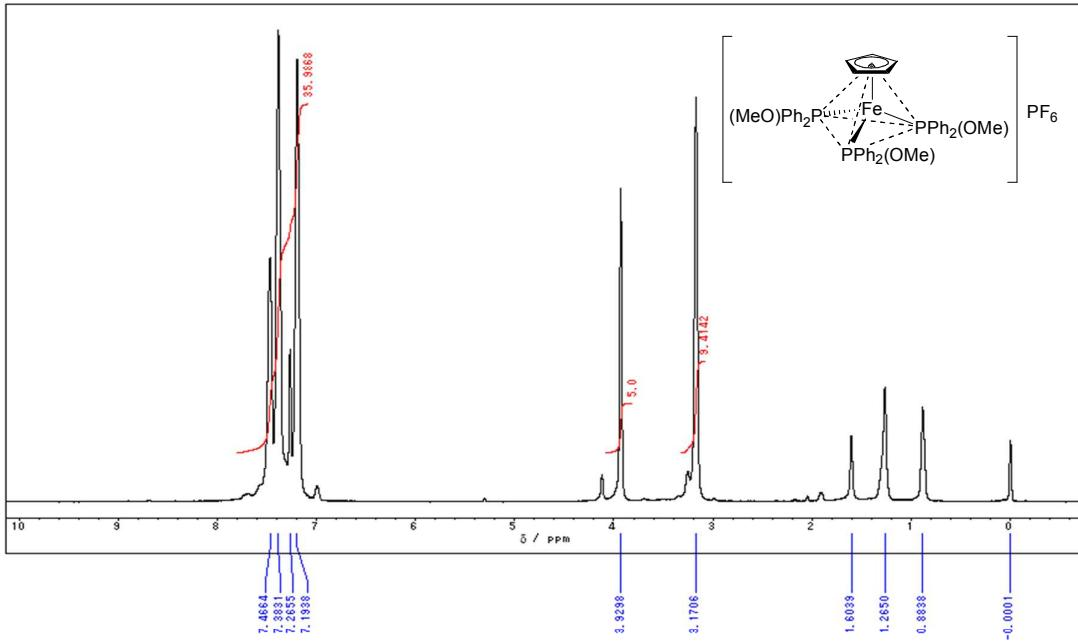
**Figure S26-1.**  $^1\text{H}$  NMR Spectrum of  $[\text{CpFe}\{\text{PPh}_2(\text{OMe})\}_3]\text{PF}_6$  in  $\text{CDCl}_3$  at 293 K.
