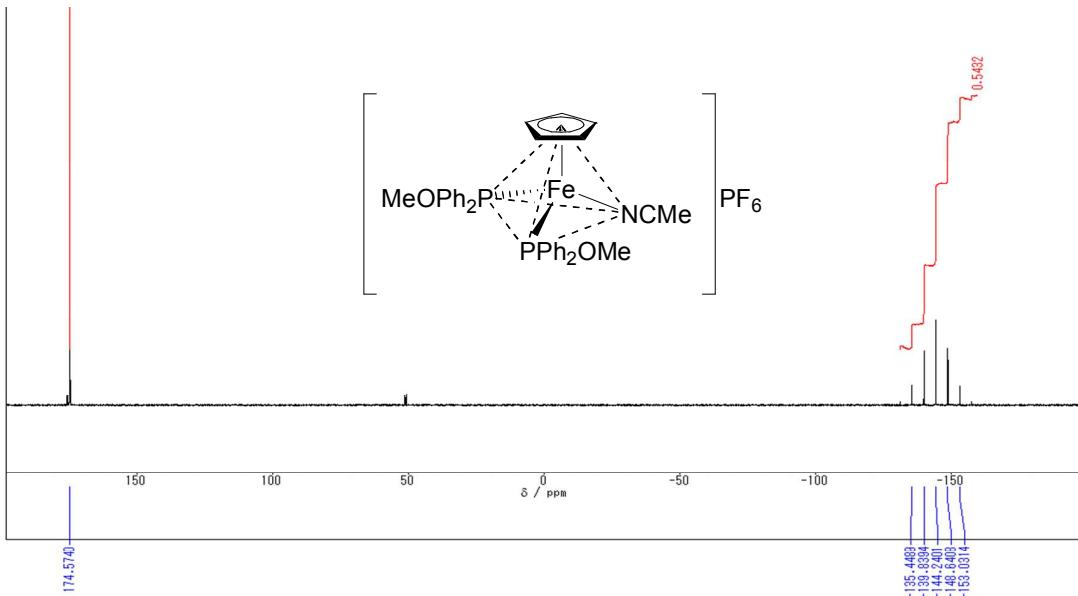
**Figure S25-3.**  $^{31}\text{P}\{^1\text{H}\}$  NMR Spectrum of  $[\text{CpFe}\{\text{PPh}_2(\text{OMe})\}_2\text{NCMe}]\text{PF}_6$  in  $\text{CDCl}_3$  at 293 K.
