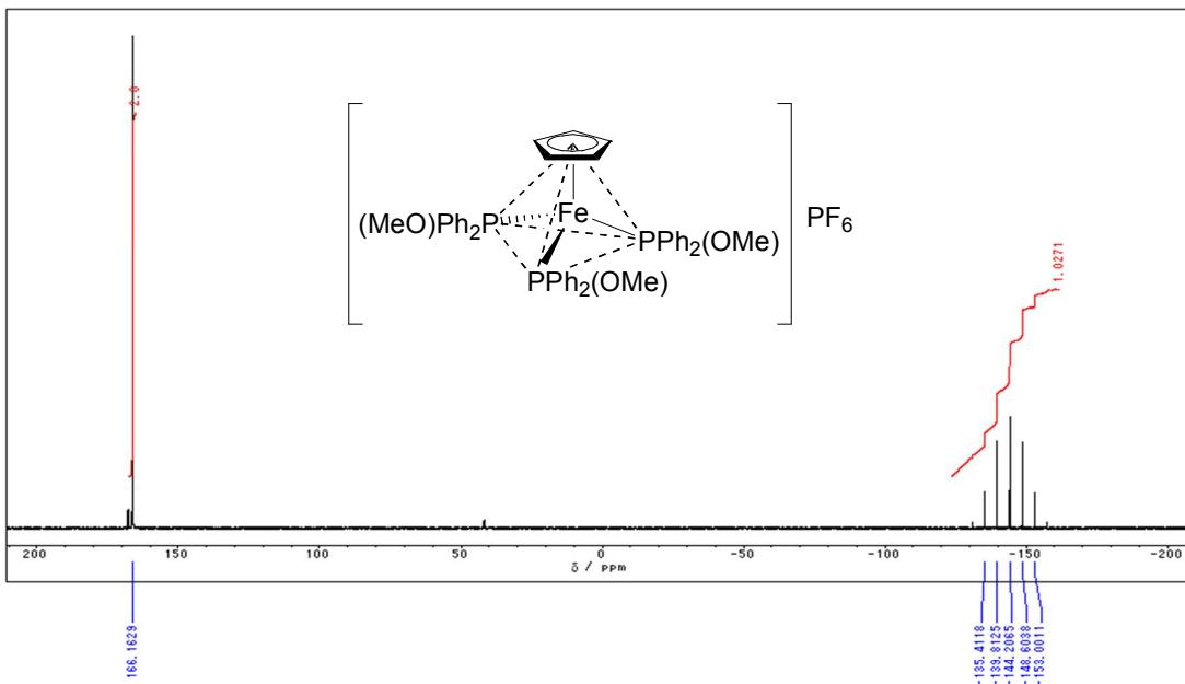
**Figure S26-3.**  $^{31}\text{P}\{^1\text{H}\}$  NMR Spectrum of  $[\text{CpFe}\{\text{PPh}_2(\text{OMe})\}_3]\text{PF}_6$  in  $\text{CDCl}_3$  at 293 K.
