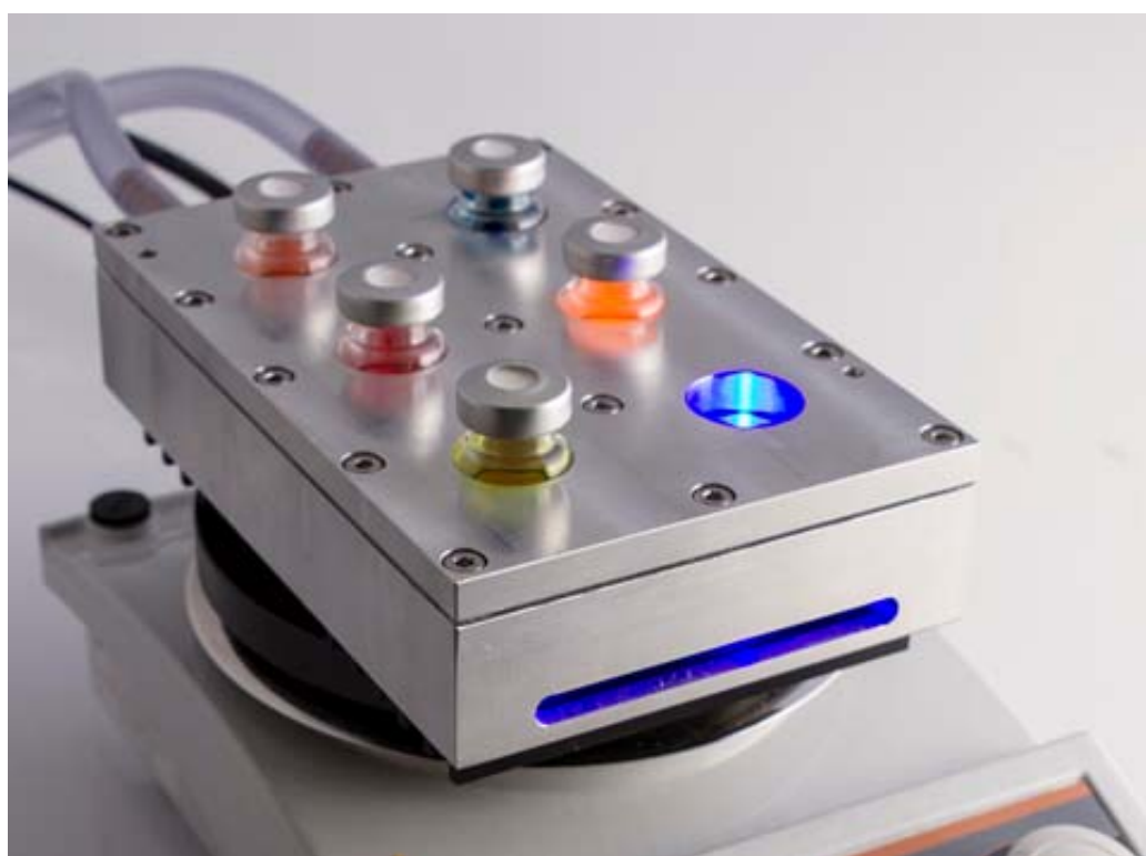
Figure S1. Photograph of the photochemical reaction setup. The reaction vials (5 mL crimp cap vials) were illuminated from the bottom side with blue LEDs ( \lambda_{\text{ex}} = 455 (\pm 15) nm) and cooled (to maintain the reaction temperature of 25 °C) from the side using custom-made aluminum cooling blocks connected to a thermostat. Photograph reproduced with permission of Burkhard König.
