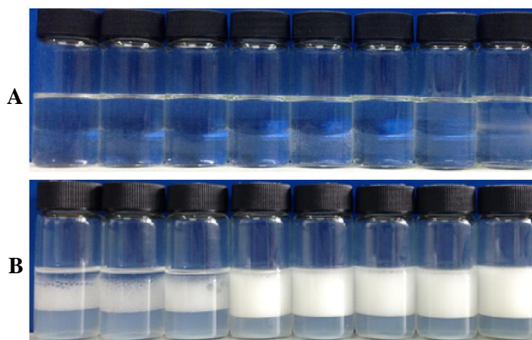
Figure S6. Photographs of toluene-in-water (7 mL/7 mL) emulsions stabilized by (A) C_{12}E_3 alone and (B) mixtures of 0.5 wt.% silica nanoparticles and C_{12}E_3 at different concentrations taken 1 week after preparation at room temperature ( 22 \pm 2 °C). [C_{12}E_3] /mM in toluene from left to right: 0.1, 0.3, 0.6, 1, 3, 6, 10 and 30.
