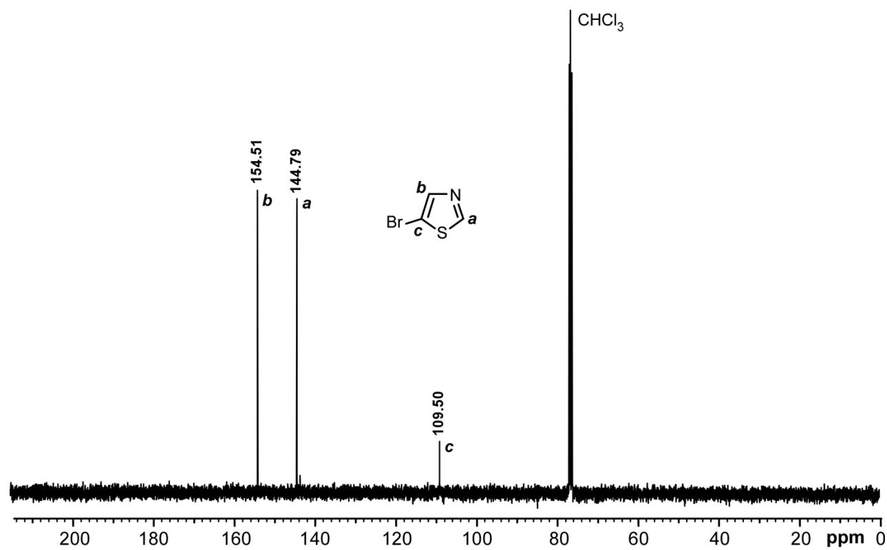
**Figure S8.**  $^{13}\text{C}$  NMR spectrum of **4** in  $\text{CDCl}_3$
