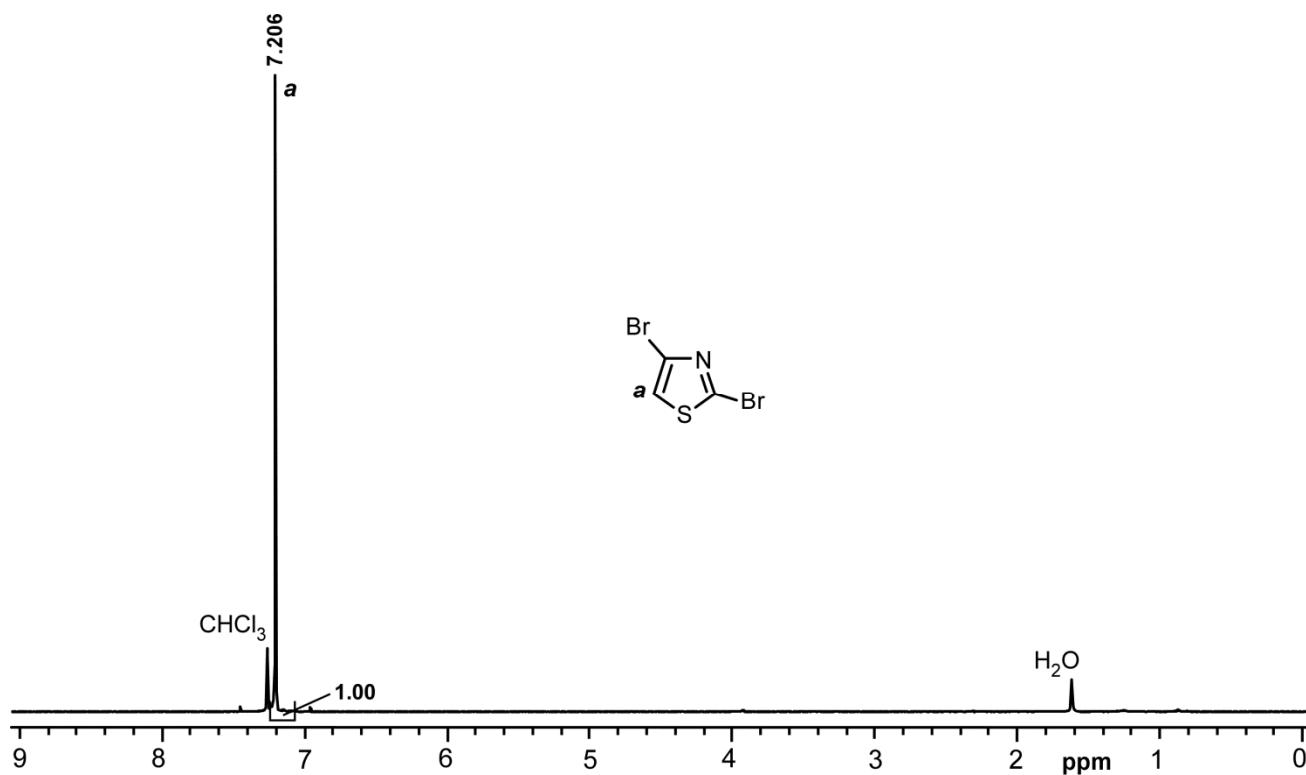
**Figure S9.**  $^1\text{H}$  NMR spectrum of **5** in  $\text{CDCl}_3$
