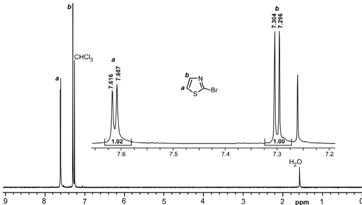
**Figure S1.**  $^1\text{H}$  NMR spectrum of **1** in  $\text{CDCl}_3$
