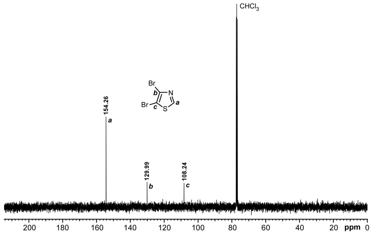
**Figure S15.**  $^{13}\text{C}$  NMR spectrum of **8** in CDCl<sub>3</sub>
