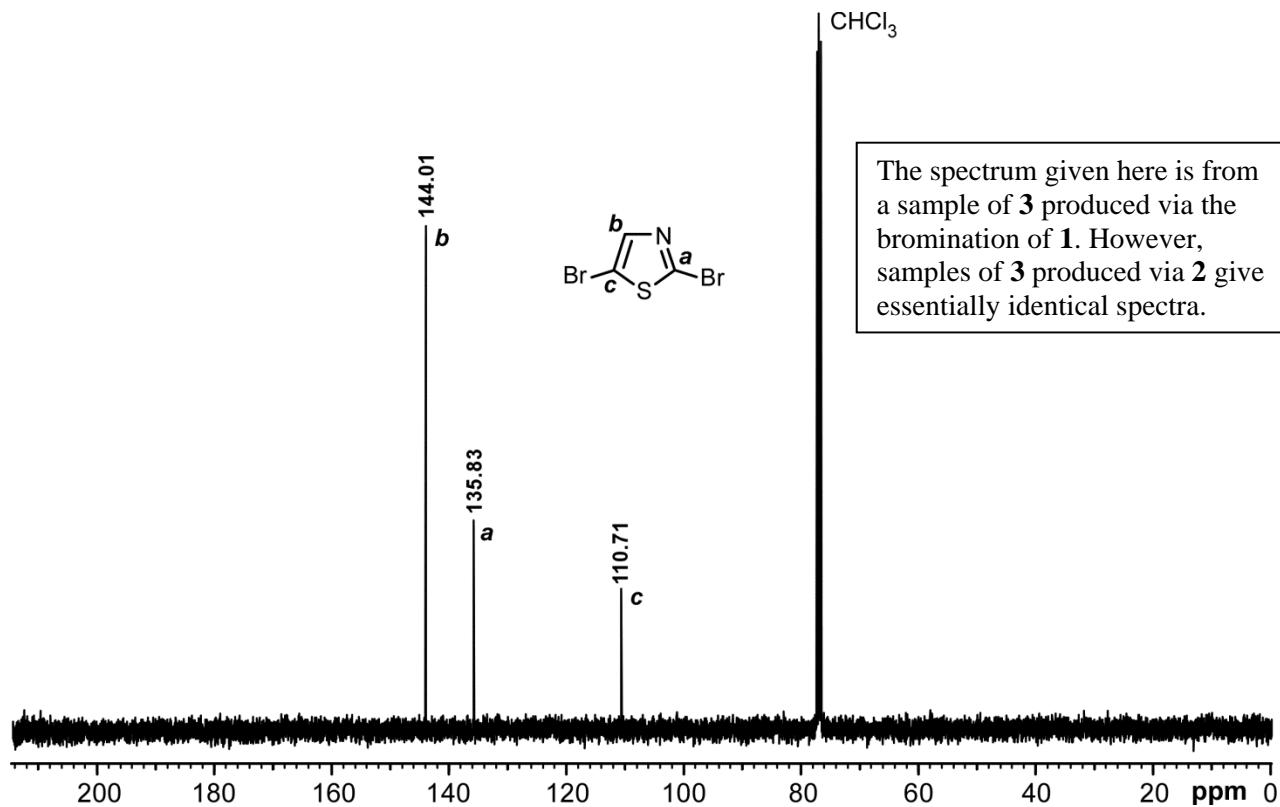
**Figure S6.**  $^{13}\text{C}$  NMR spectrum of **3** in  $\text{CDCl}_3$
