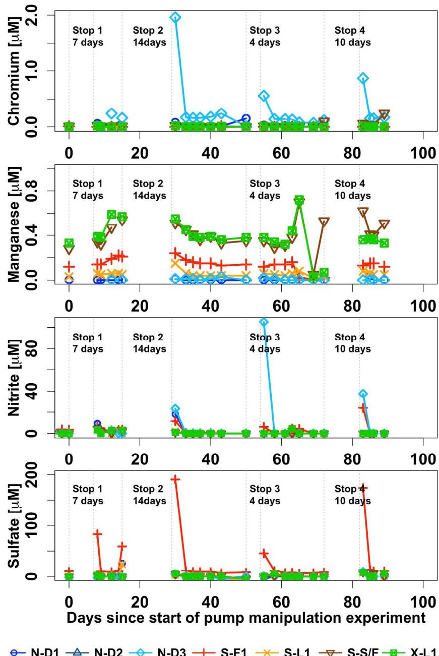
**Figure SI-7** Effluent chromium and manganese concentrations in the denitrifying columns.
