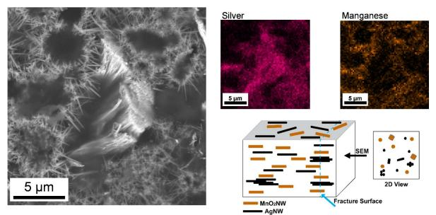
Figure S2: SEM image of the fracture surface of 2.0vol% AgNW/1.0vol% MnO<sub>2</sub>NW/PMMA hybrid
