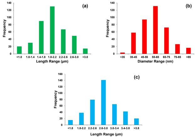
Figure S1. Size distribution for synthesized nanowire: (a)  $MnO_2NW$ - length distribution, (b)  $MnO_2NW$ -
