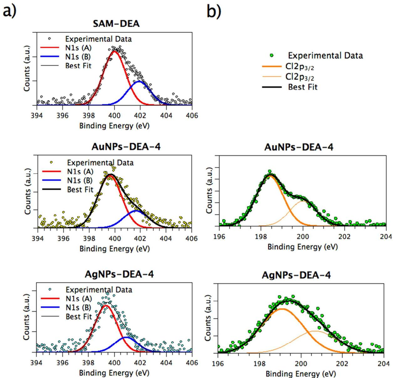
**Figure SI-8.** XPS a) N1s and b) Cl2p spectra collected on SAM-DEA, AuNPs-DEA-4 and AgNPs-DEA-4 samples.
