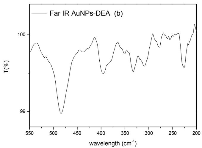
Figure SI-3: Far-IR spectrum (film from chloroform) of AgNPs-DEA (a) and AuNPs-DEA (b)
