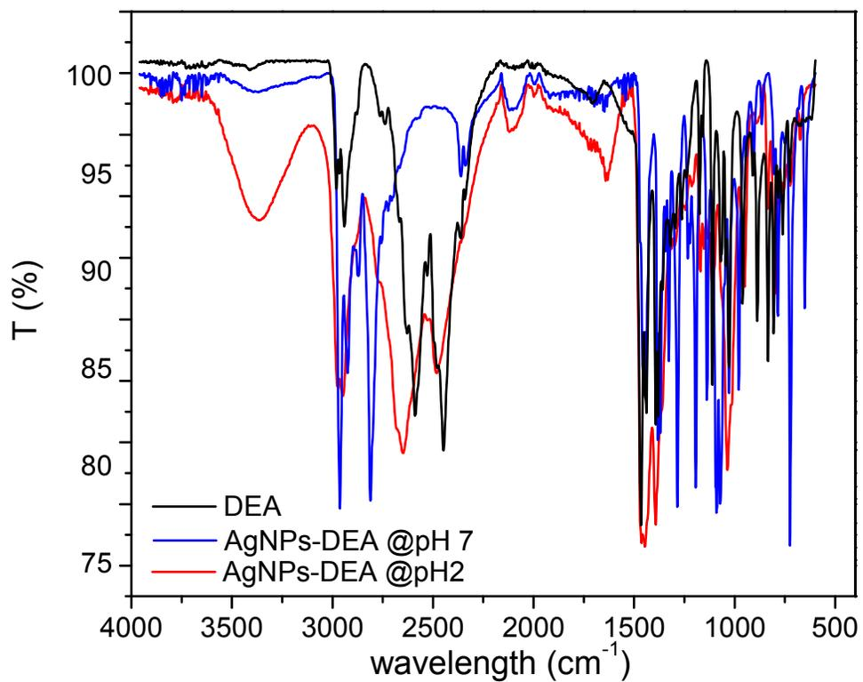
*Figure SI-2:ATR spectra of AgNPs-DEA film from water at pH 2 and 7 compared with DEA powder.*
