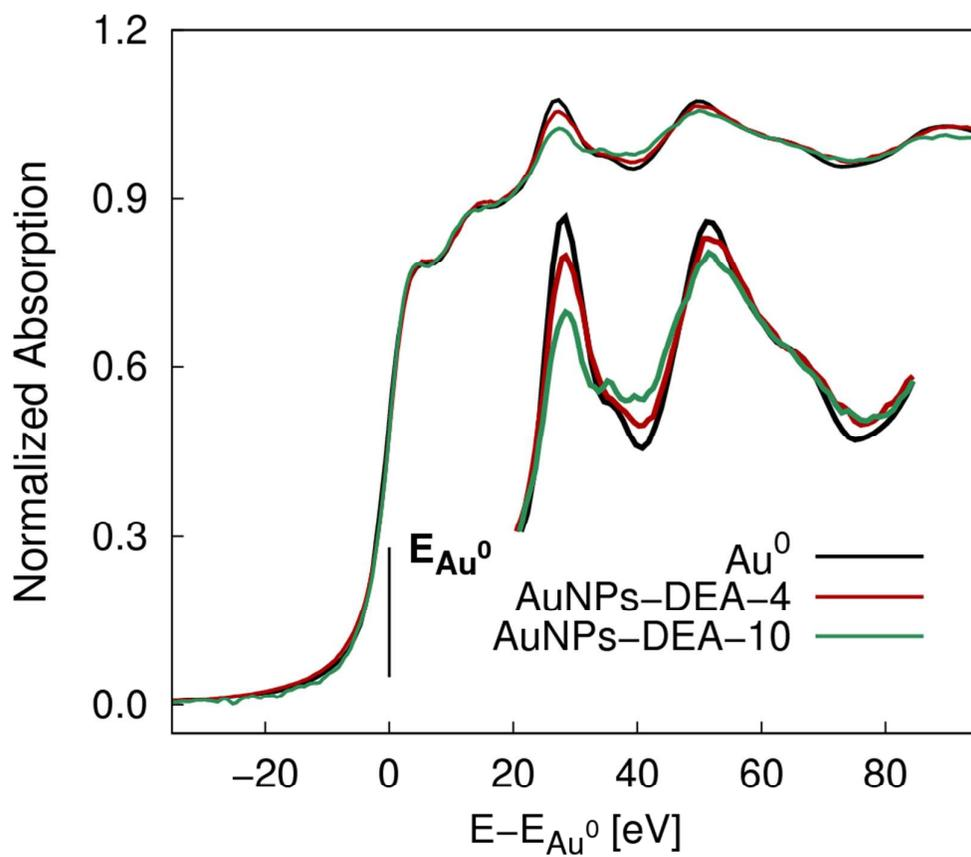
Fig.SI 9.: The Au-LIII normalized absorption spectra for Au-reference foil (black) and AuNPs-DEA samples (red and green curves). The fine structure oscillations progressively decrease (see inset curves) accordingly to the decreasing NPs size.
