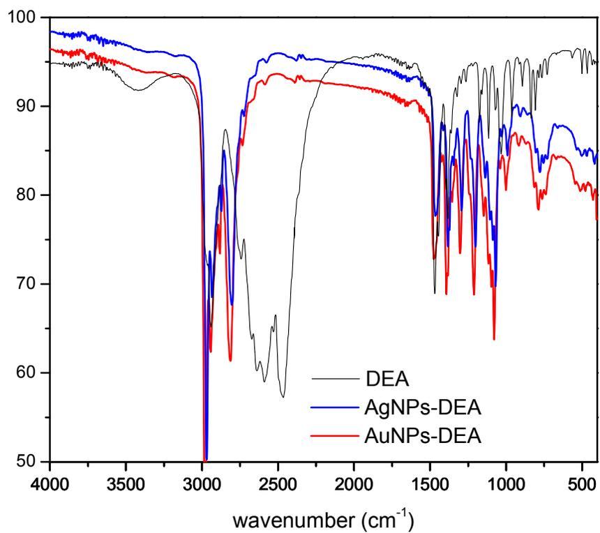
Figure SI-1: FT-IR spectra (film) of AuNPs-DEA and AgNPs-DEA samples at pH 7; compared with DEA thiol.
