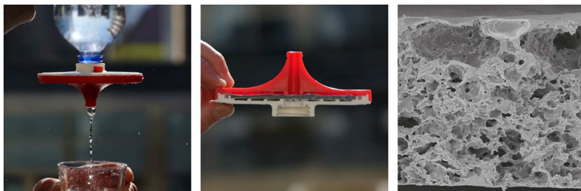
Figure: Photograph of the commercial unit in use with a PET bottle. The cross-section of the filter housing shows an activated carbon filling as well as a thin polymer membrane. The scanning electron microscopy image on the right shows a cross-section of the filter membrane itself.
