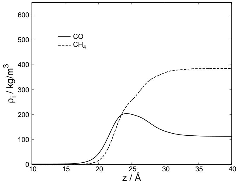
Figure 1: Density profiles of the vapor-liquid interface at  $x_{\text{CO}}^{\text{liq}} = 0.0202$  and  $p = 0.6 \text{ bar}$ .
