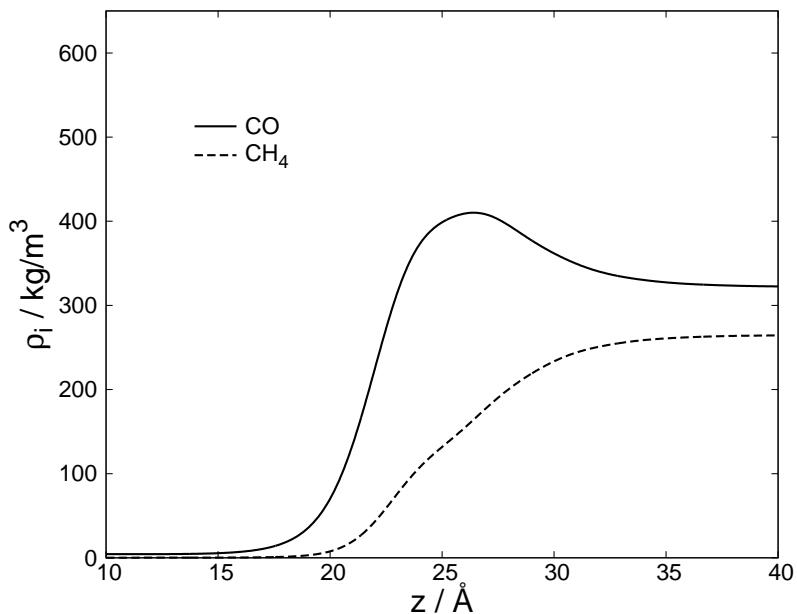
Figure 2: Density profiles of the vapor-liquid interface at  $x_{\text{CO}}^{\text{liq}} = 0.4104$  and  $p = 1.2 \text{ bar}$ .
