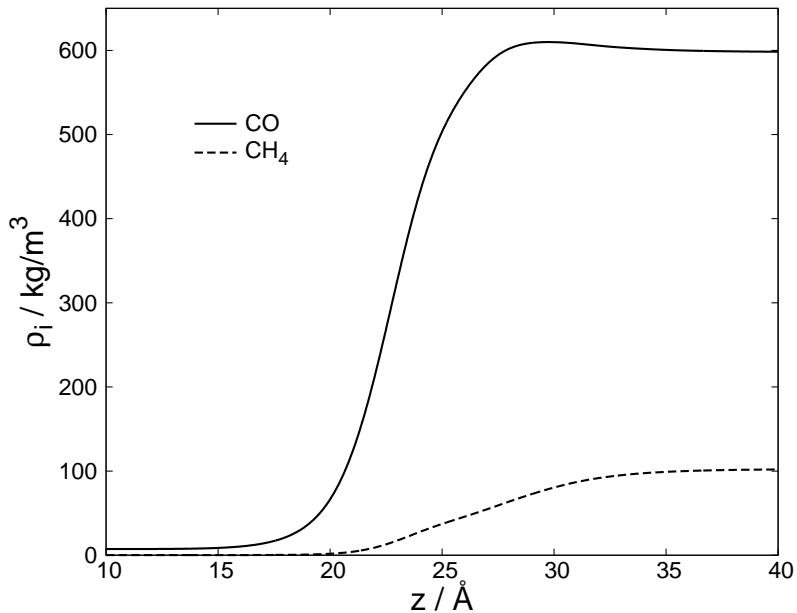
Figure 3: Density profiles of the vapor-liquid interface at  $x_{\text{CO}}^{\text{liq}} = 0.770$  and  $p = 1.9 \text{ bar}$ .
