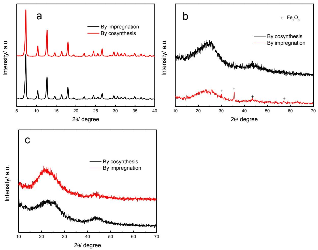
**Figure. S6** XRD patterns of FeZIF-0.84 precursor prepared by co-synthesis and impregnation method(a); C-FeZIF-900-0.84 before acid leaching(b) and after acid leaching(c)
