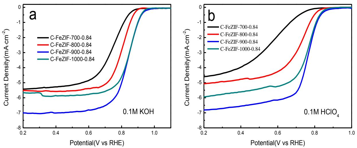
**Figure. S5** ORR curves of C-FeZIF-0.84 in  $0.1\text{M KOH}$ (a) and  $0.1\text{M HClO}_4$ (b) at different pyrolysis temperatures
