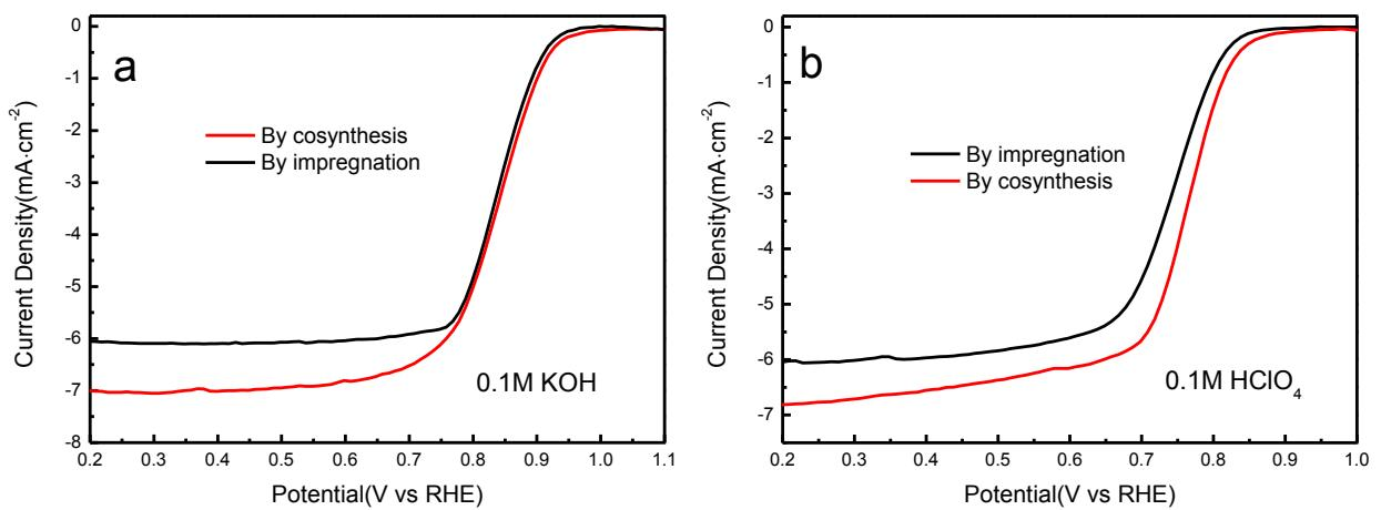
**Figure. S8** ORR curves of C-FeZIF-900-0.84 in 0.1M KOH(a) and 0.1M  $\text{HClO}_4$ (b) prepared by cosynthesis and impregnation method
