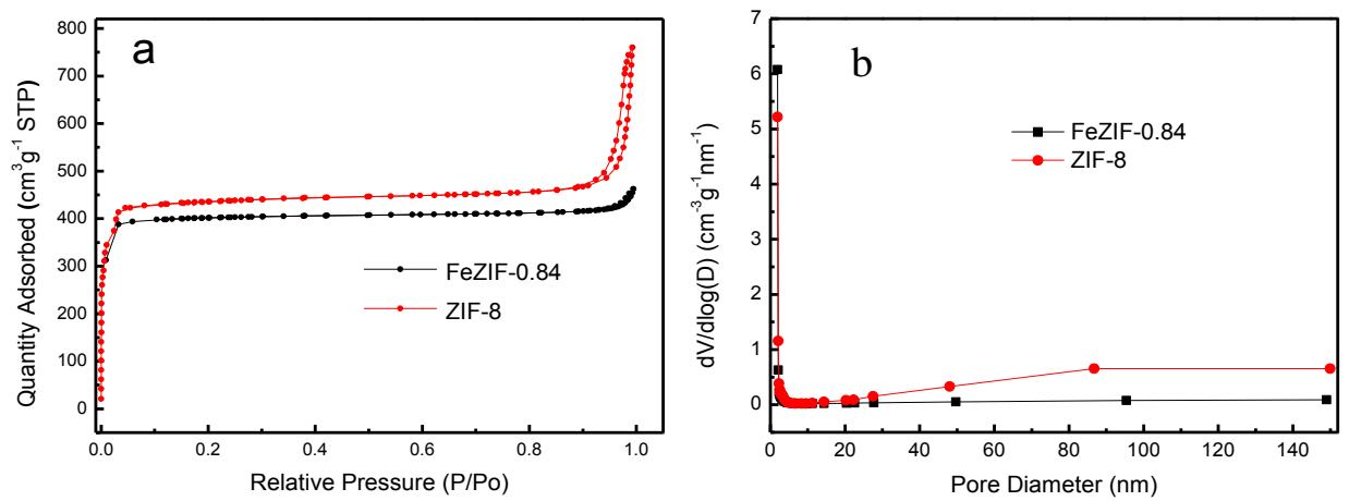
**Figure. S4** N<sub>2</sub> adsorption and desorption isotherms(a) and pore size distributions(b) of ZIF-8 and FeZIF-0.84
