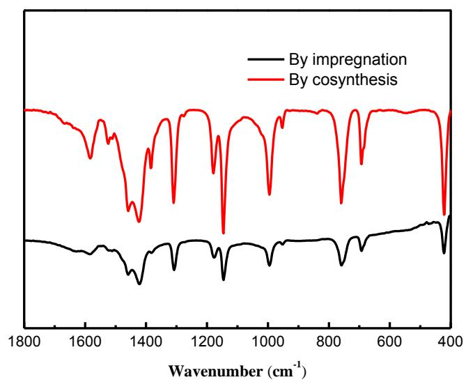
**Figure. S7** FTIR spectra of FeZIF-0.84 precursor prepared by co-synthesis and impregnation method
