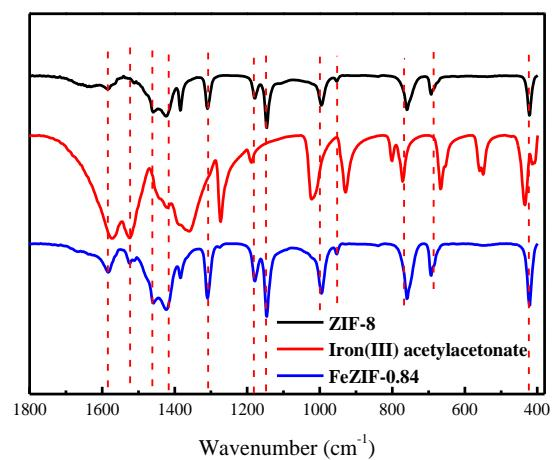
**Figure. S2** FTIR spectra of the ZIF-8, Iron(III) acetylacetone, FeZIF-0.84
