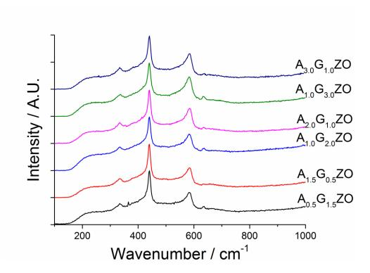
Figure S1. Raman spectra of the six representative AGZO samples. With regards to the observed dominating modes, the [E2 (high) – E2 (low)] mode of ZnO appeared at 331 cm $^{-1}$ , the E2 high signal appeared at 438 cm $^{-1}$ , the E1(LO) mode appeared at 581 cm $^{-1}$ . Additionally, a small peak appeared at 632 cm $^{-1}$ , caused by the presence of  $Ga_2O_3(A_g \text{ mode})$ . This peak was observed more strongly for those samples with more gallium in the precursor solutions.
