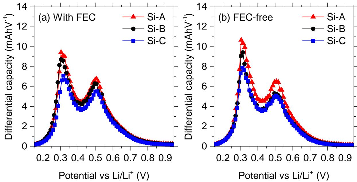
**Figure S9.** Differential capacity ( $dQ/dV$ ) plots of the Si NP/Li half cells using (a) electrolyte with FEC; and (b) electrolyte without FEC at 0.5 C rate, showing the absence of the expected characteristic c-Li<sub>15</sub>Si<sub>4</sub> peak at 0.45 V vs. Li/Li<sup>+</sup>.
