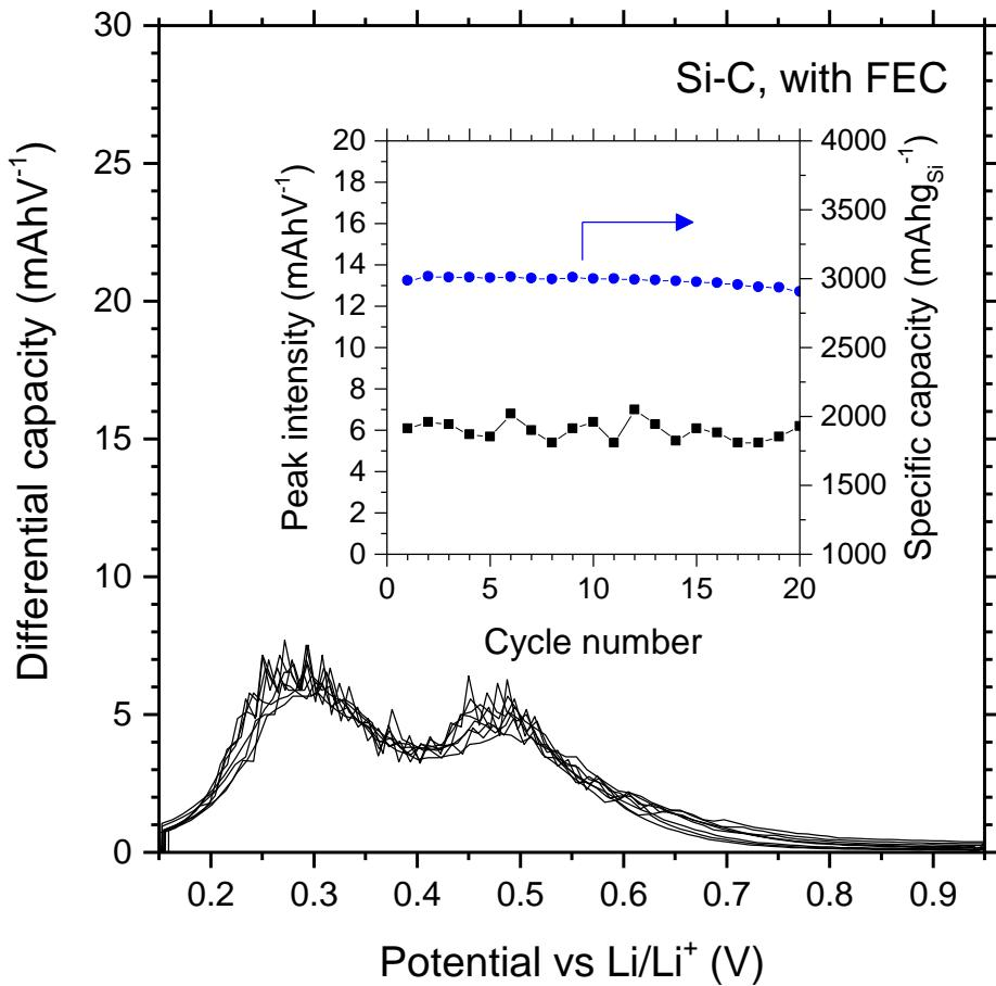
**Figure S7.** Evolution of differential capacity ( $dQ/dV$ ) plot of the Si-C NP/Li half cell during cycling under 0.1 C rate with FEC (inset shows the specific charge capacity as well as the intensity of the c- $\text{Li}_{15}\text{Si}_4$  peak at 0.45 V vs.  $\text{Li}/\text{Li}^+$  as a function of cycle number).
