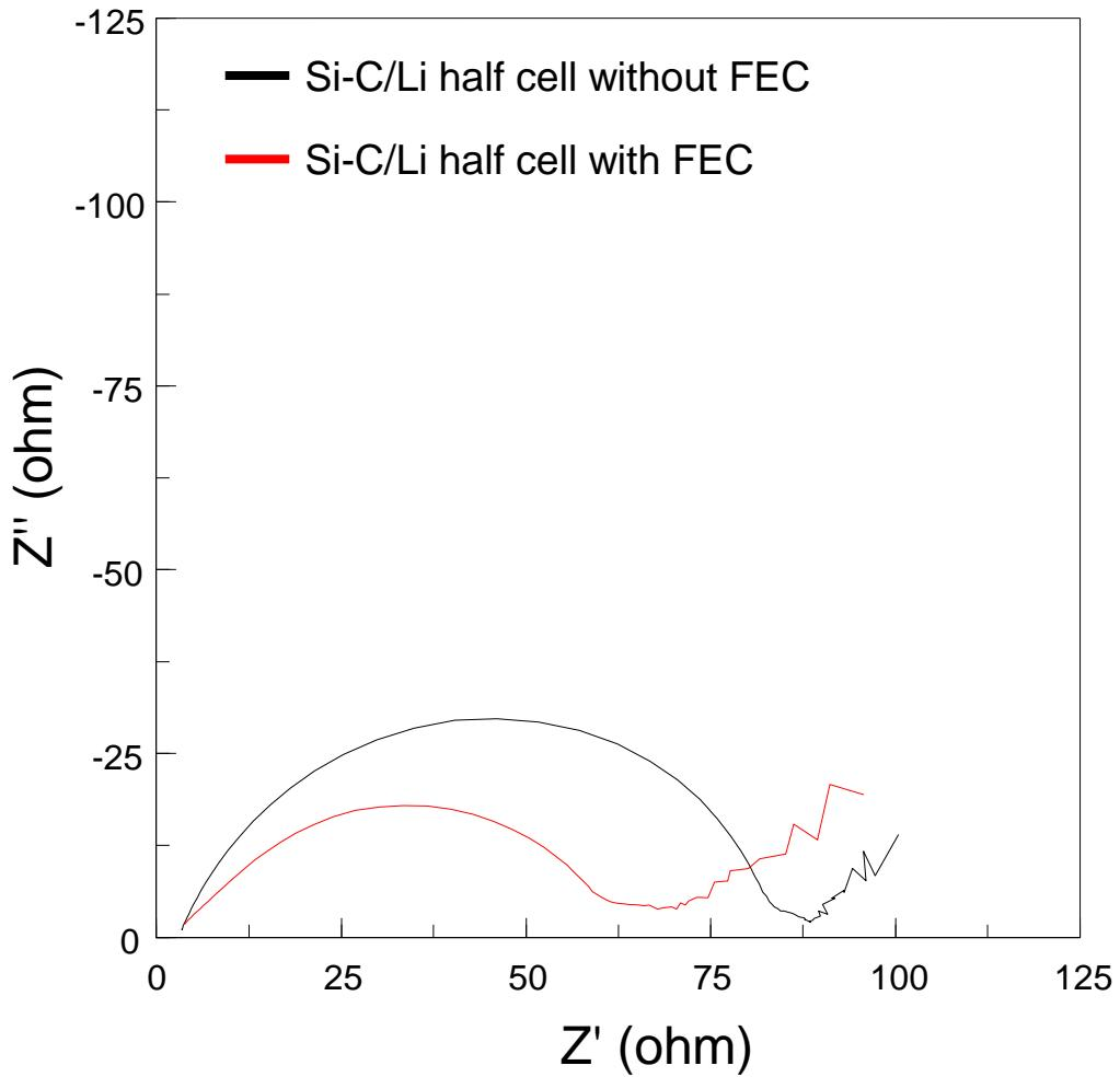
**Figure S10.** Nyquist plots of Si-C/Li half cells with and without FEC at 0 V vs. Li/Li<sup>+</sup> (2<sup>nd</sup> discharge, Frequency range = 100 kHz to 0.01 Hz, 10 mV amplitude).
