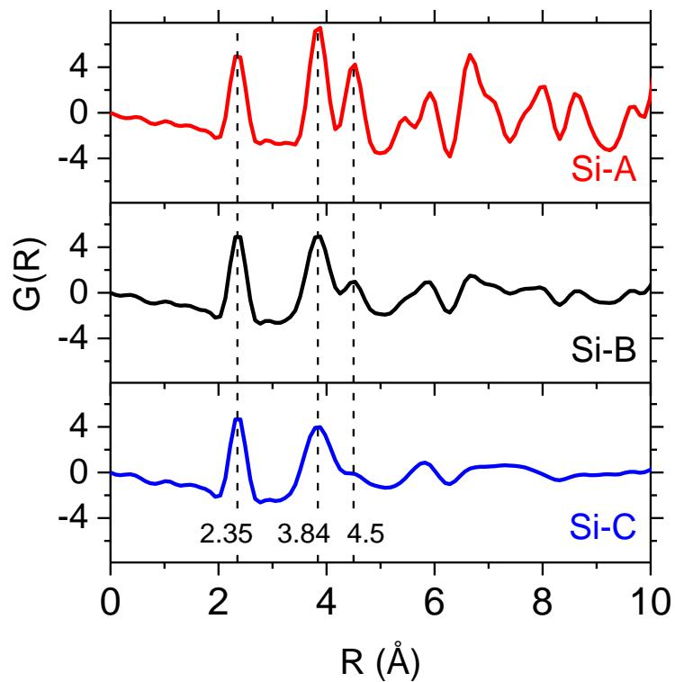
**Figure S1.** Pair distribution functions of Si-A, Si-B, and Si-C. The dashed lines correspond to the 1<sup>st</sup>, 2<sup>nd</sup>, and 3<sup>rd</sup> coordination shell Si-Si distances in a Si diamond matrix.
