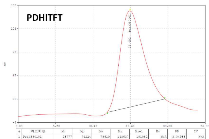
Figure S1-16 Gel permeation chromatogram of the PDHITFT polymer run in chloroform solution
