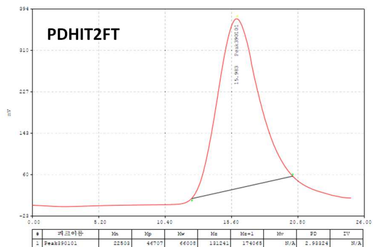
Figure S1-17. Gel permeation chromatogram of the PDHIT2FT polymer run in chloroform solution
