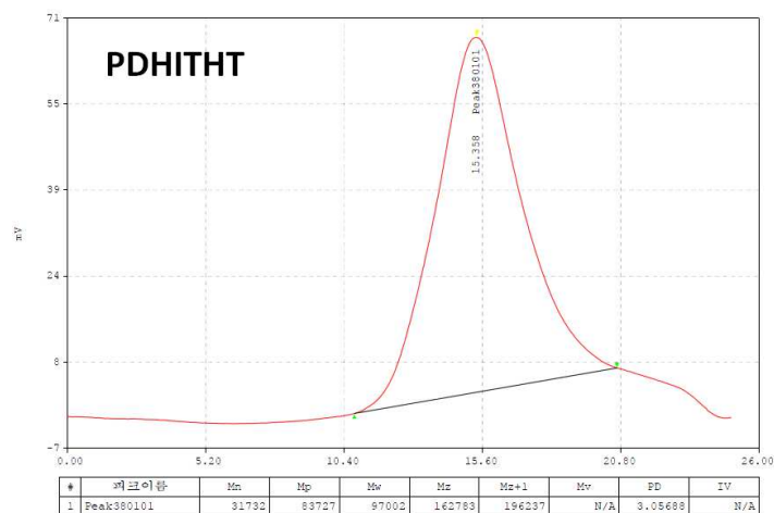
Figure S1-15 Gel permeation chromatogram of the PDHITHT polymer run in chloroform solution
