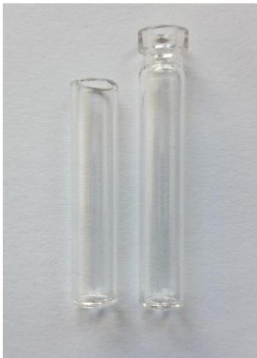
**Figure S3.** Left: vial after removal of the top part; right: crimped vial.
