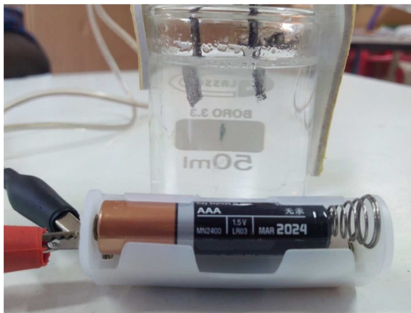
Figure S11: A snapshot taken the during operation of two electrode water electrolyser that consists the \text{Ni}_3\text{Se}_4 nanoassemblies on Ni foam as both anode and cathode while powered with an AAA alkaline battery of optimum voltage output of 1.5 V.
