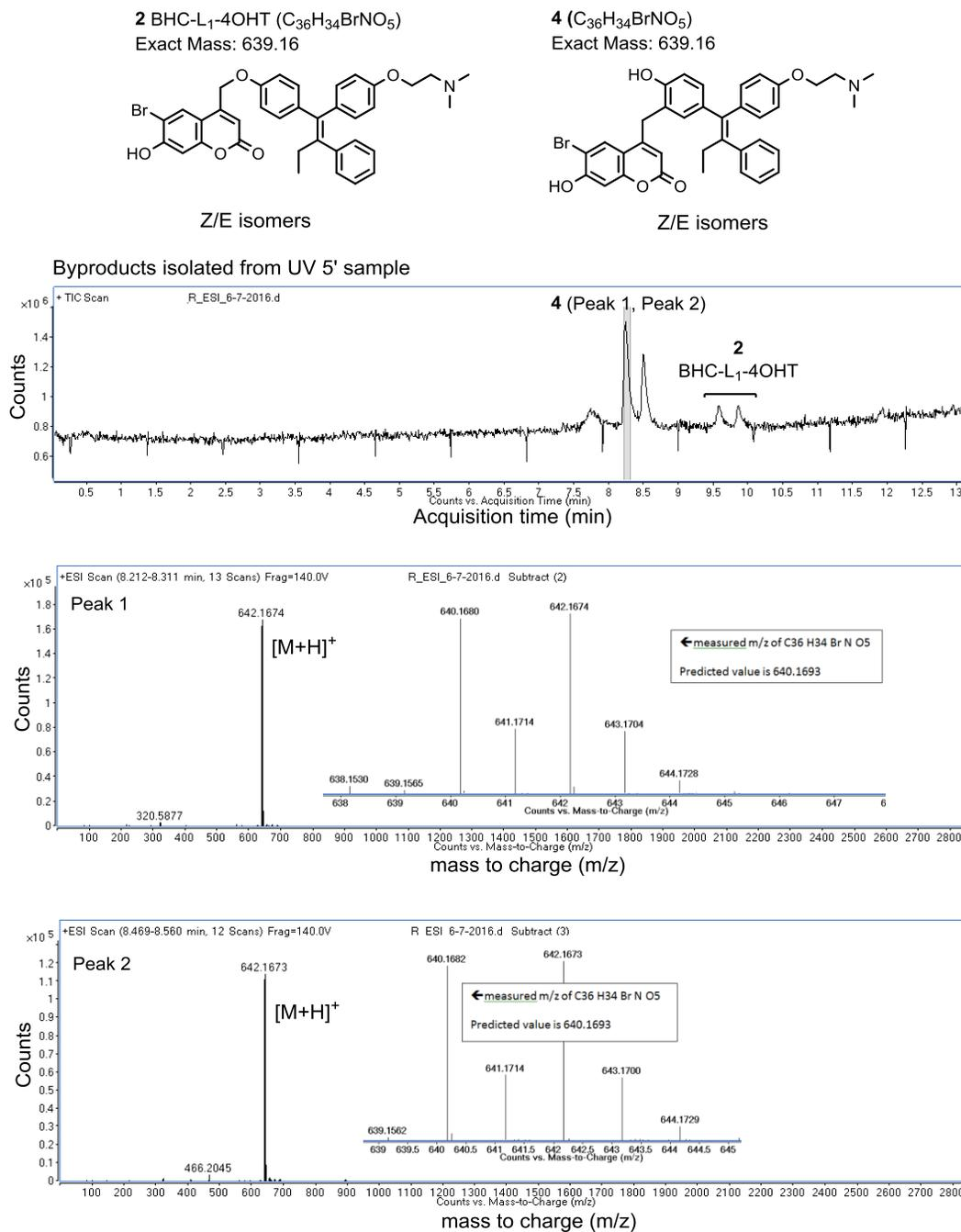
**Figure S8.** (Top) Structures of **2** BHC-L<sub>1</sub>-4OHT and **4** the proposed photo-Claisen byproduct, and (Bottom) LC-MS analysis of the isolated byproduct (the same sample shown in Figure 2C; bottom), confirming that both peak 1 and peak 2 (Z/E isomers) are identical in their mass as anticipated from **4**.
