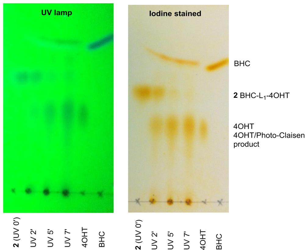
**Figure S7.** TLC analysis of reaction products after photolysis (2, 5 and 7 min; 365 nm) of **2** BHC-L<sub>1</sub>-4OHT, showing the lack of resolution between free 4OHT and the photo-Claisen byproduct. Visualization method: UV lamp (left), iodine staining (right).
