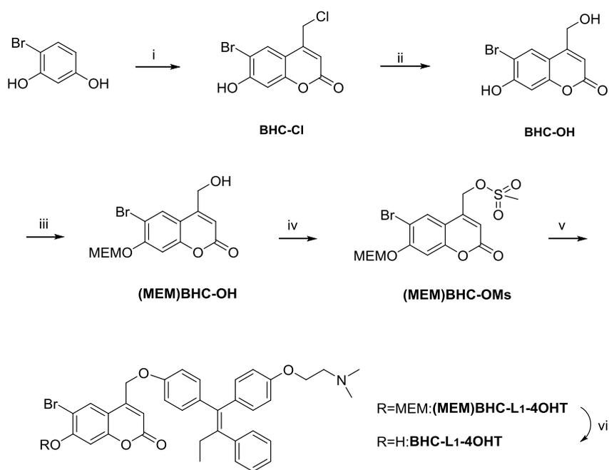
*reagents and conditions:* i) Ethyl 4-chloroacetoacetate, methanesulfonic acid; ii) H<sub>2</sub>O, reflux, 24 h; iii) 2-methoxyethoxymethyl chloride (MEMCl), DIPEA, CH<sub>2</sub>Cl<sub>2</sub>; iv) methanesulfonyl chloride, DIPEA, CH<sub>2</sub>Cl<sub>2</sub>; v) 4OHT, K<sub>2</sub>CO<sub>3</sub>/Cs<sub>2</sub>CO<sub>3</sub>, THF; vi) CF<sub>3</sub>CO<sub>2</sub>H, CH<sub>2</sub>Cl<sub>2</sub>.
