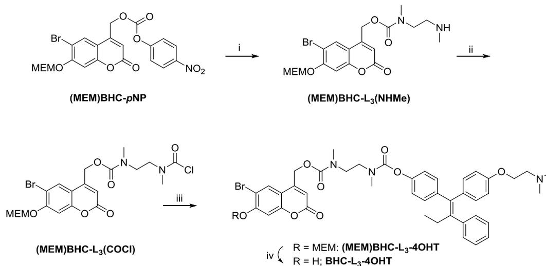
reagents and conditions: i) *N,N'*-dimethylethane-1,2-diamine, DIPEA, THF; ii) triphosgene, DIPEA, CH<sub>2</sub>Cl<sub>2</sub>; iii) 4OHT, DIPEA, DMAP, CH<sub>2</sub>Cl<sub>2</sub>; iv) TFA, CH<sub>2</sub>Cl<sub>2</sub>, rt
