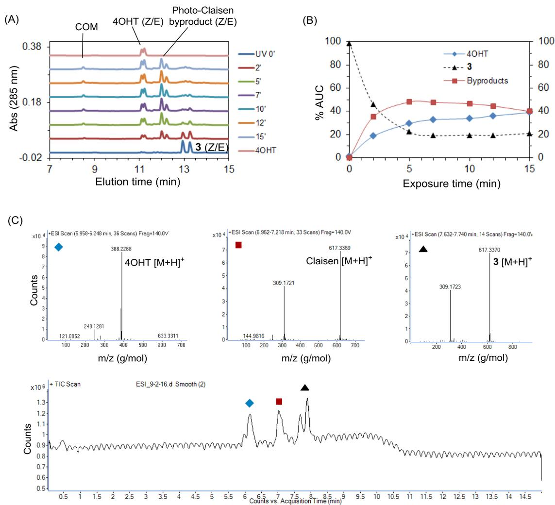
**Figure S10.** Mechanism of photolysis of **3** COM-L<sub>1</sub>-4OHT that accounts for the release of 4OHT in addition to generation of the photo-Claisen byproduct. (A) Overlaid UPLC traces acquired after photolysis of **3** (78  $\mu$ M in 20% v/v aq. methanol); (B) A plot of area under curves (%AUC) for 4OHT, **3** and the byproduct as a function of exposure time; (C) LC-MS analysis after 10 min photolysis of **3**, confirming the masses anticipated for 4OHT and the photo-Claisen byproduct.
