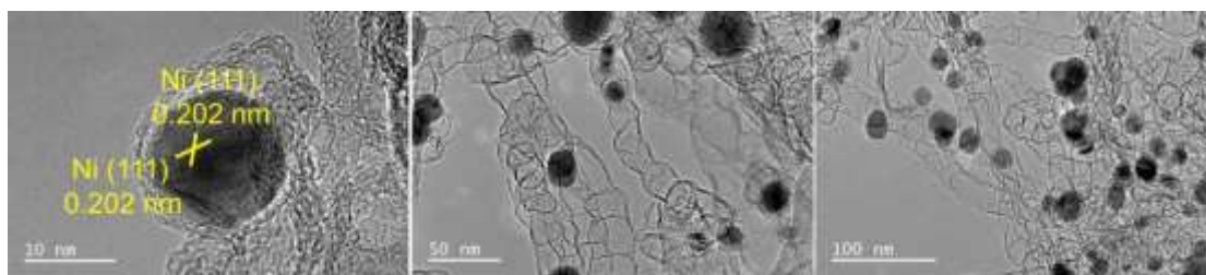
Figure S17. HRTEM images of NiO x @BCNTs treated via H 2 -TPR process under 400 °C.
