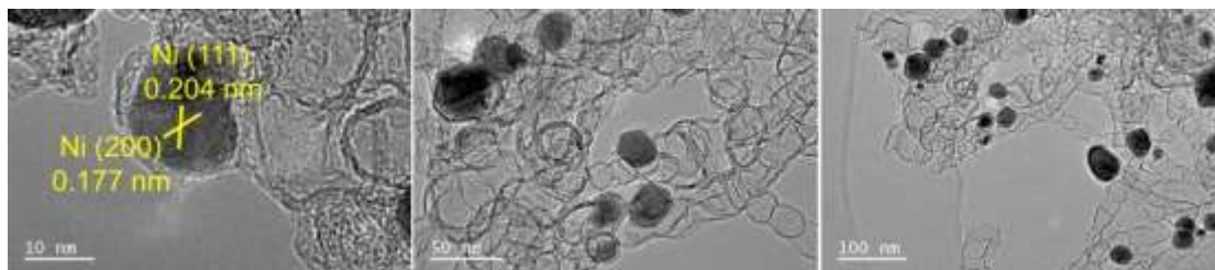
Figure S20. HRTEM images of NiO x @BCNTs treated via H 2 -TPR process under 750 °C.
