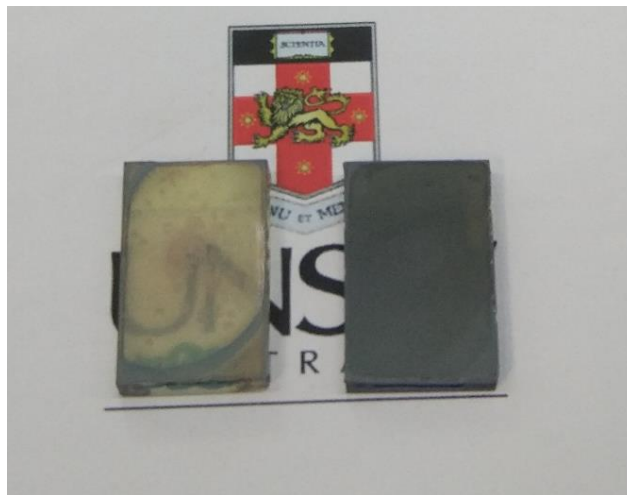
Figure S1. A photo of \text{FA}_{0.95}\text{Rb}_{0.05}\text{PbI}_3 (left) and \text{FA}_{0.95}\text{Cs}_{0.05}\text{PbI}_3 (right) annealed at 110^\circ\text{C} for 20 min.
