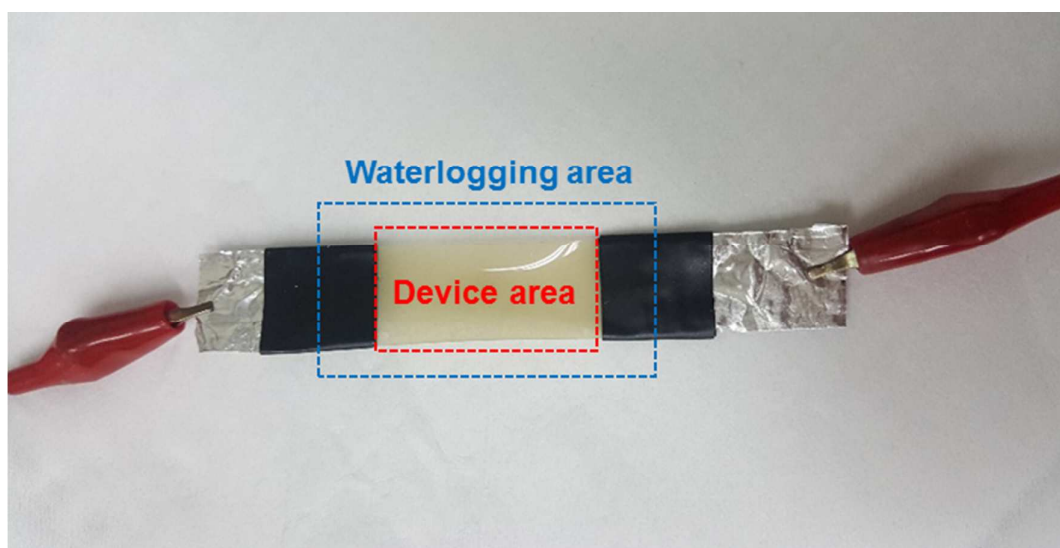
Figure S12. Sealing of the AgNW electrodes from exposure to water.
